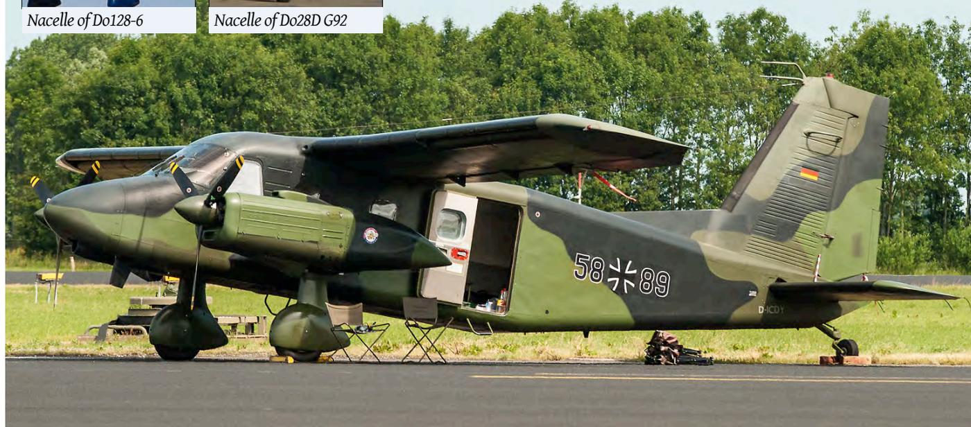
Although the Dornier 28D has a similar arrangement as the earlier variants, it looks more like a different aircraft: it has a much larger fuselage. Most were built as piston version, like this former Luftwaffe Do28D-2 D-ICDY. The small photos show the nacelles of two turboprop versions. (Leeuwarden, 21 June 2008)
