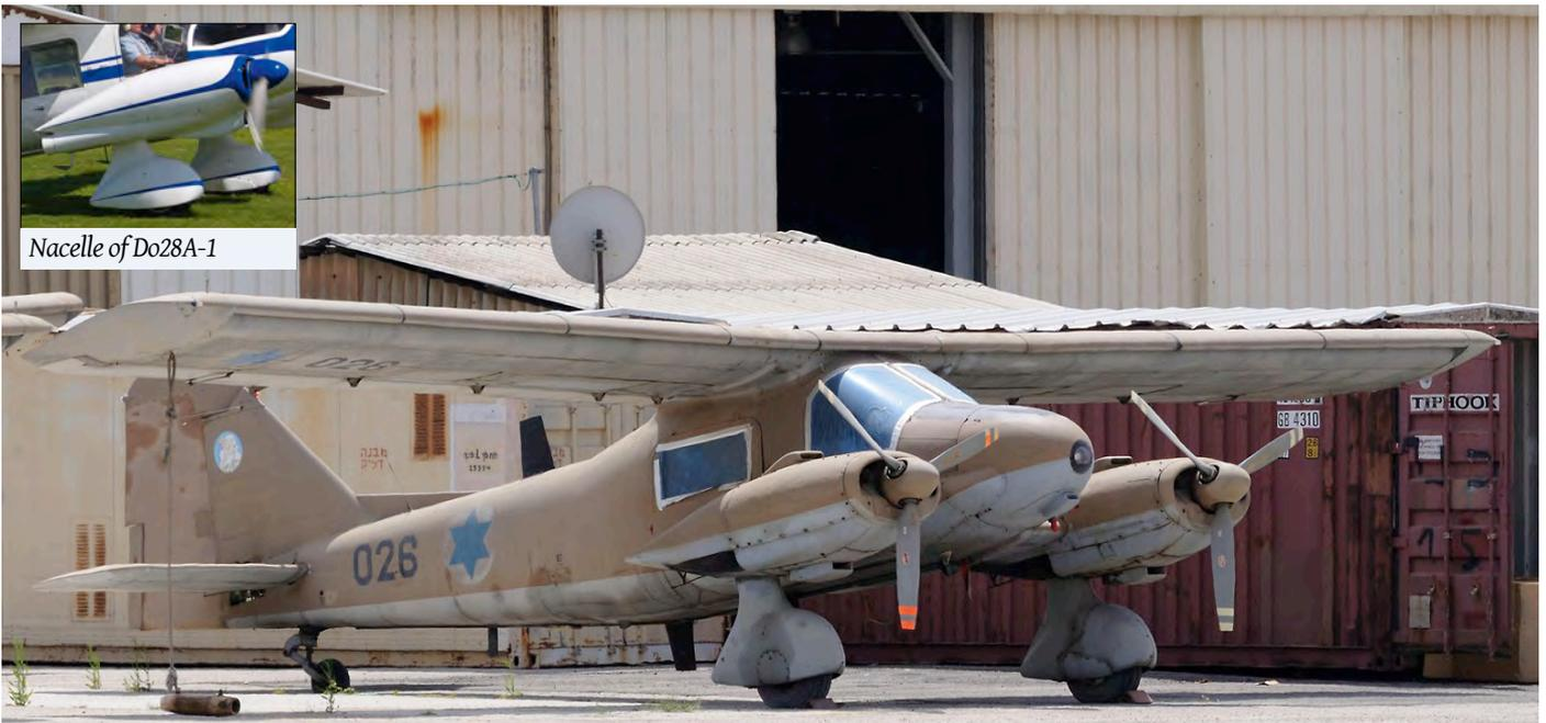
The Dornier 28 is essentially a twin version of the Dornier 27. If you are familiar with that aircraft you will probably recognise the fuselage and wing shape. New are the two piston engines attached to the forward fuselage with struts. Shown here is Do28A-1 026 of the Israeli Air Force. The inset shows the different location of the oil cooler on the Do28A-1. (Sde Dov, 5 May 2008, Erwin van Dijkman)
