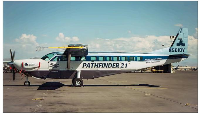
Conversion specialist Soloy fitted the 208B with two PT6As driving a single prop. To balance the higher weight of the engine pack, the fuselage was lengthened by nearly two metres primarily behind the wing. Just one was built before the programme was halted. (photo above of N5010Y at North Las Vegas in October 1998)
