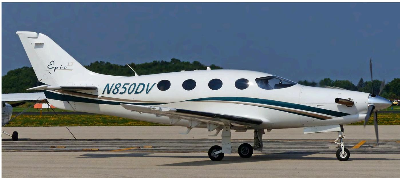
The Epic LT has so far been produced as a home-built, but the E1000 is to be the certified version of the single engine turboprop. It resembles the Kestrel JP10 (formerly Farnborough F1) very much, so compare the photos to see that the difference is in the cockpit windows and engine exhausts. (N850DV, Fond du Lac (WI), 31 July 2014, Dave Hopkins)
