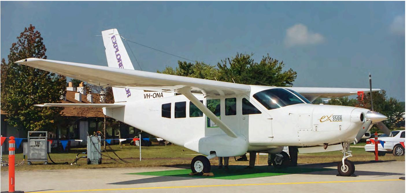
Another single engine aircraft in the class of the Cessna Caravan: the Explorer series. The 350R VH-ONA shown here is the piston version, the turboprop version is called the Explorer 500T. So far production is limited to a few aircraft. Look at the retractable gear to distinguish it from the other high wing single engine aircraft.
