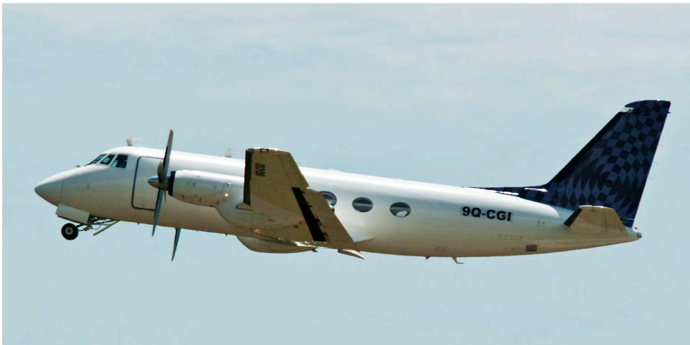
Compared to other bizprops described in this article the Gulfstream I is by far the largest. It is only because it has been developed as a bizprop from the start that it is not categorised as a commuter. The large Gulfstream style cabin windows, as seen on 9Q-CGI, make it stand out easily between the commuters. (anonymous)
