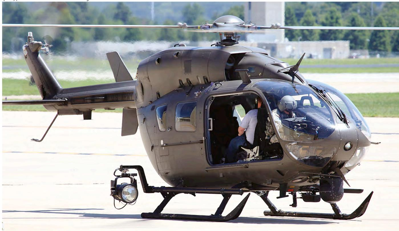
About three-and-a-half years after delivery of the first UH-72A, the S&S MEP was introduced in active service. The two most eye-catching features of this mission equipment package are the FLIR underneath the forward fuselage and the searchlight mounted on the right-hand side of the helicopter. Both are excellently visible on this picture. (12-72251, Fort Smith RAP, Arkansas, 13 August 2014, Coert van Breda)
