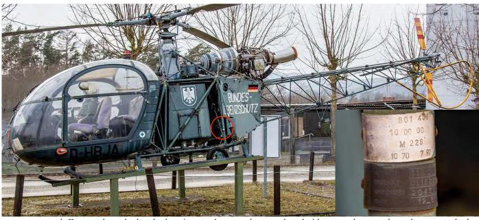
Grenzmuseum Schifflersgrund at Asbach Sickenberg (previously reported as at Bad Sooden) has a Bundesgrenzschutz Alouette 2 on display. This (77+28)/D-HBJA should have construction number 2017, however it is marked as 2047 on the plate. The plate with the construction number can be found on the tubular horizontal frame on the left side of the helicopter. See red circle and insert. (25 March 2021, Wolfgang Birmes)
