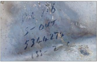
Serial BK716 still readable on the inside of a panel from the starboard outer engine. (Authors)
