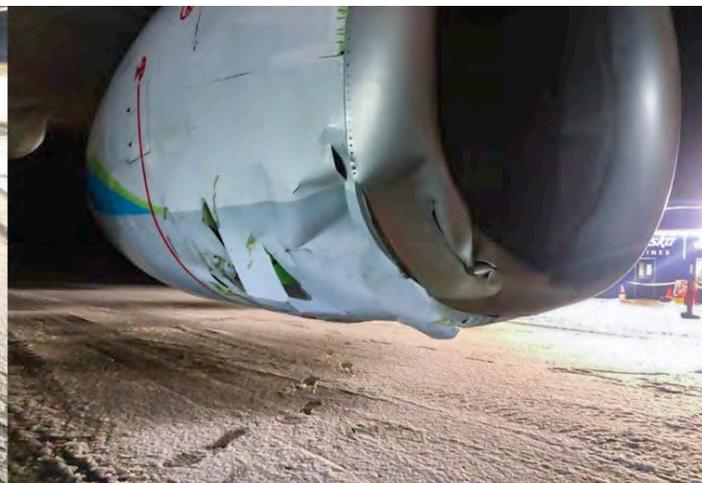
Scheduled to fly Anchorage (AK) - Cordova (AK) - Yakutat (AK) - Juneau (AK) - Seattle-Tacoma (WA), on 14 November 2020, Alaska Airlines flight AS66 had to cancel the last two sectors after it hit a bear during landing at Yakutat's runway 11. While damage to Boeing 737 N615AS was limited to the engine nacelle, the mother bear did not make it, leaving her cub behind... (Yakutat (AK), 14 November 2020, Scott McCullen)
