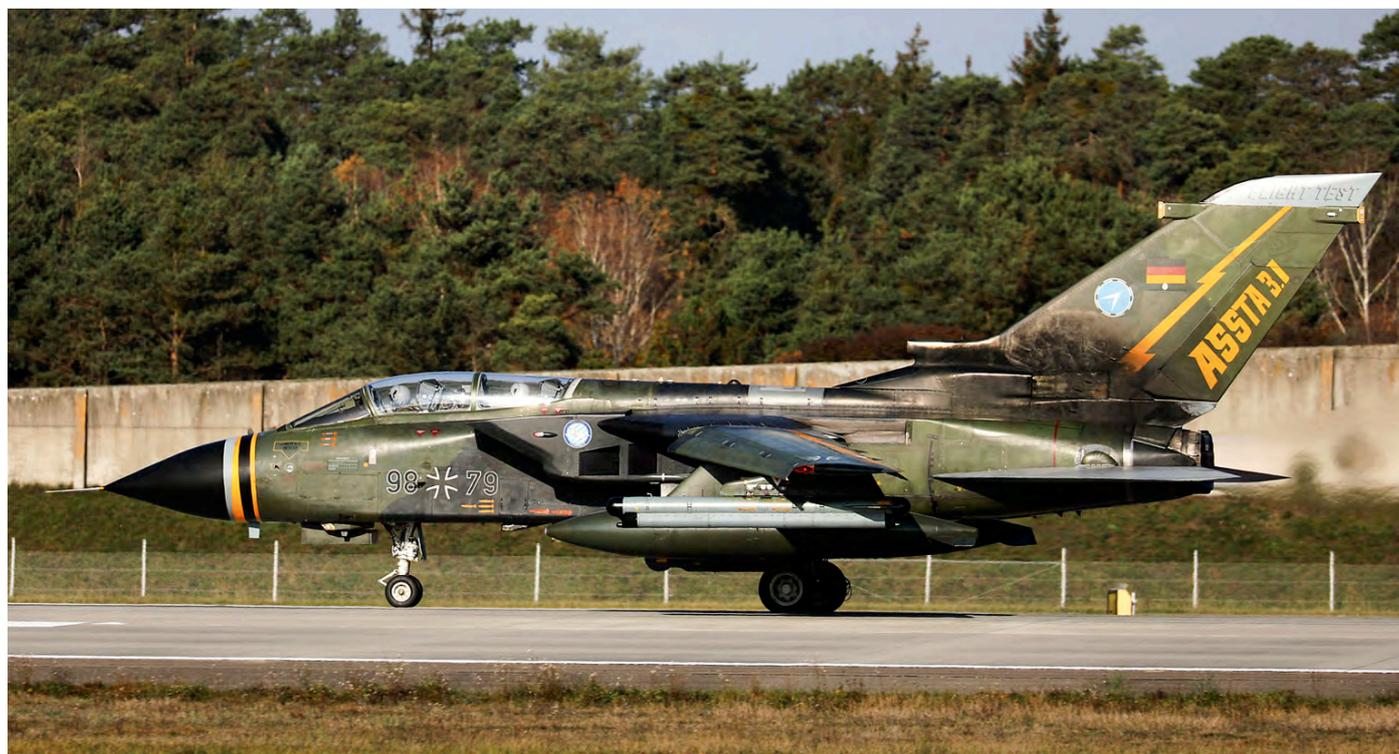
Tornado ECR test aircraft 98+79 of WTD61 was seen lining up on the runway of Manching on 5 November 2020, still wearing its ASSTA 3.1 markings but already flying for the ASSTA 4.1 upgrade program. This Tornado was actually the only German Tornado that was converted from IDS to ECR. (Josef Gietl)
