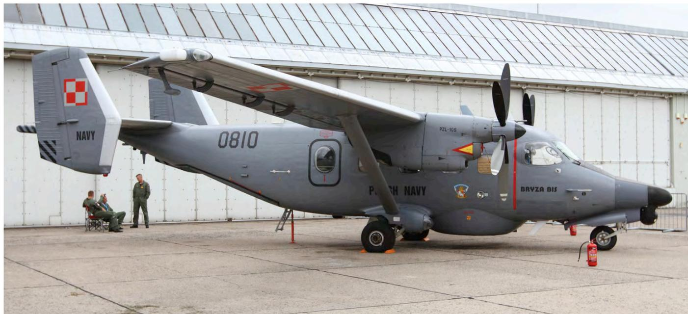
During the Radom 2018 airshow various Polish armed forces could be seen at the static display. Among the Navy participants was this M-28B Bryza 0810, showing its modified nose section after installation of a FLIR-dome. (Radom, 25 August 2018, Ian French)
