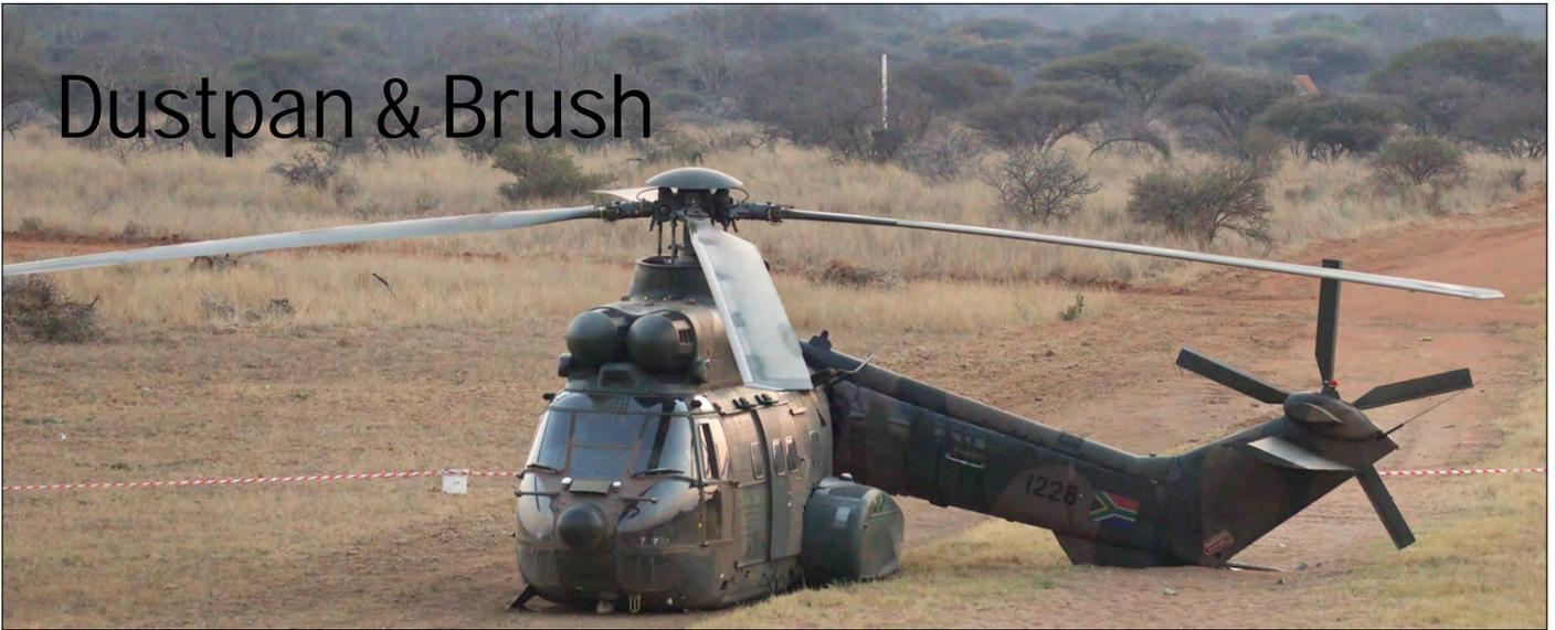
During an air show at Roodewaal, South Africa, South African Air Force Oryx 1228 touched down hard, causing the boom to snap off, as can be seen in the picture above. It appears that a phenomenon called vortex ring state was to blame for the event, which is also known as settling with power, and is a dangerous condition that may arise in helicopter flight, when a vortex ring system engulfs the rotor causing severe loss of lift. (Roodewaal, 18 September 2018, Charles Hugo)
