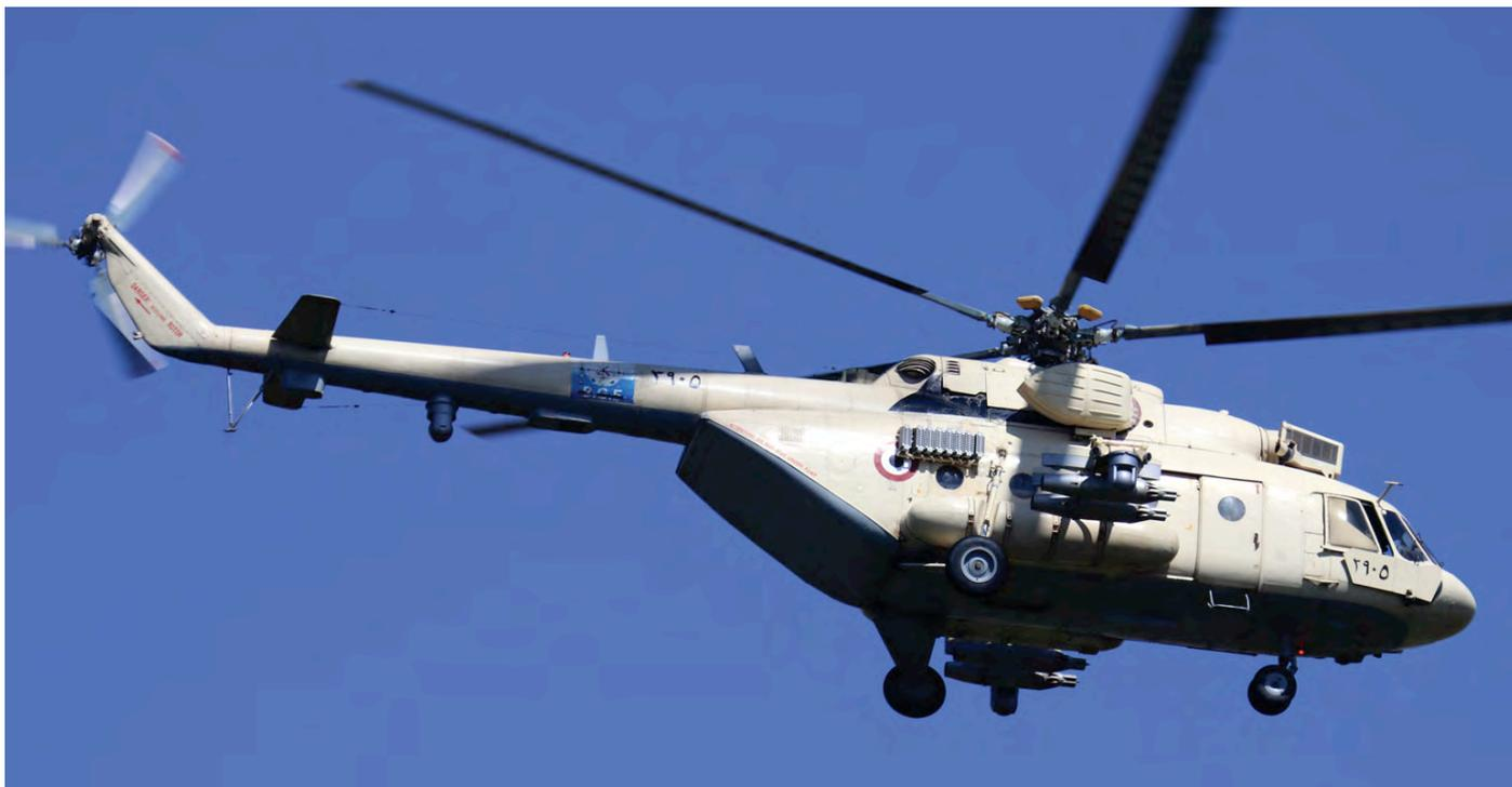
Neil Middleton presented us this tasty picture of one Egyptian Boarder Guard Force Mil Mi-17V-5 3905. Some things stand out, like the ramp at the back of the cabine and the three FLIR-cameras on the stubwing hardpoints and underneath the tail boom. (Luxor, 25 October 2017)
