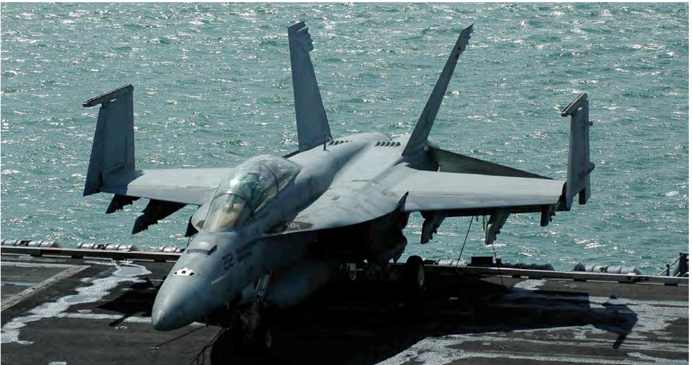
To create as much room on the flight deck as possible, aircraft are packed really close together and the ones close to the end of the flight deck are parked with their tails sticking out over the water, as can be seen with this F/A-18F. (Portsmouth-Stokes Bay, Marijn van der Burgt)
