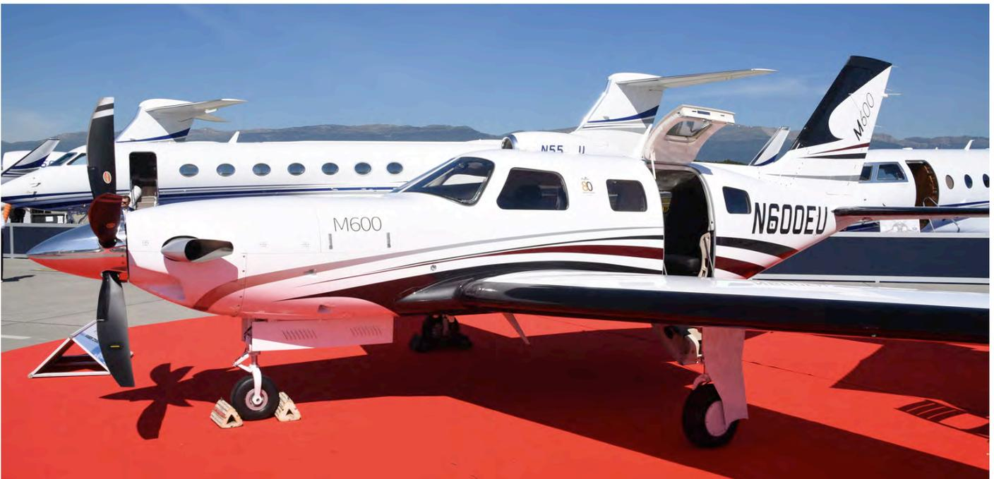
The 'M600' is a further development of the PA-46 Malibu introduced in 2015. The PA-46-600TP has a turbine engine and a pressure cabin. The wing of the aircraft is completely new designed for this model. N600EU was registered in February 2017, performed 55 demo flights and accumulated almost 100 flight hours. (Geneva, 22 May 2017, Gideon van Dijk)
