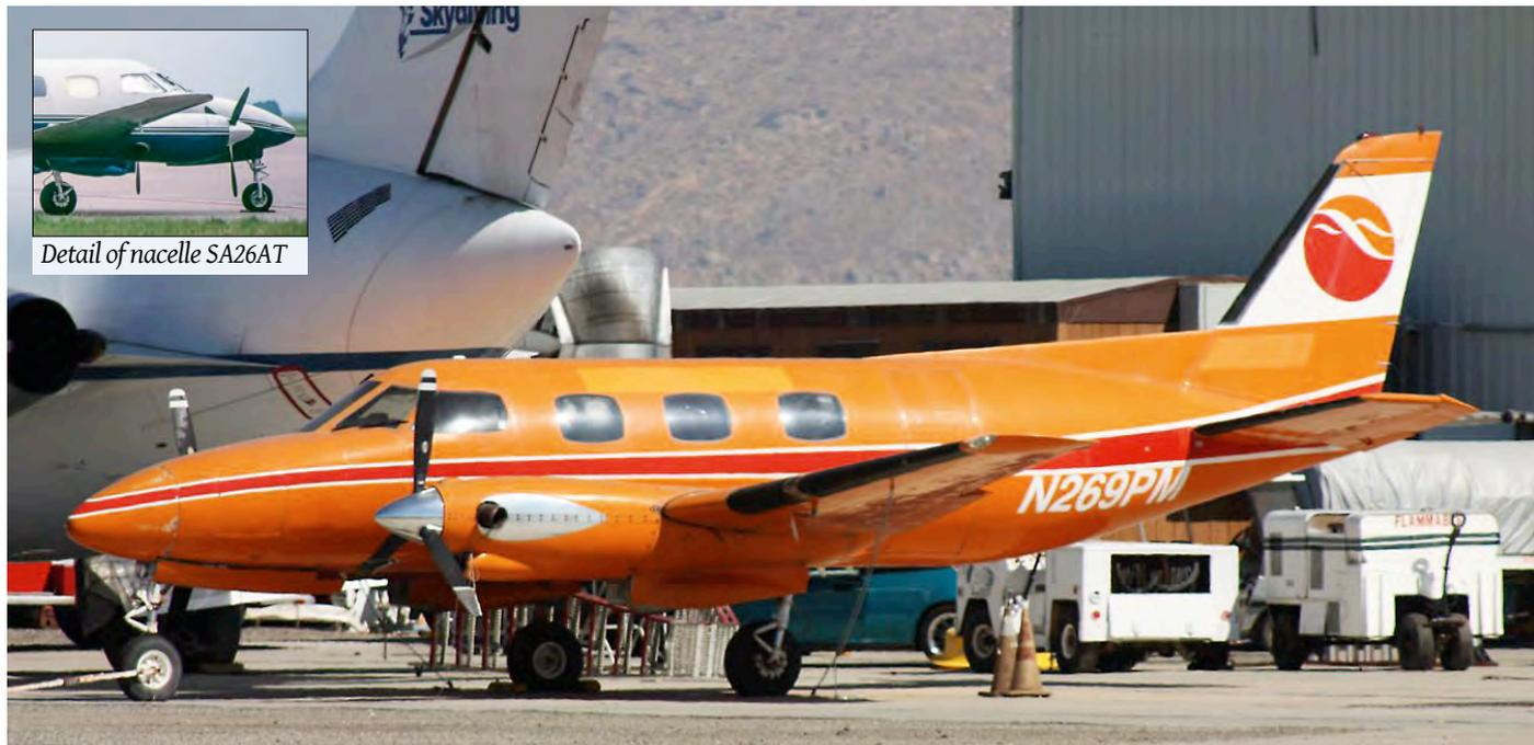
While the distinctive characteristics of the Swearingen Merlin/Metro series are visible, especially in the form of the cockpit and cabin windows, the heritage of the Beechcraft Queen Air is also apparent. Look for example at the landing gear and the tail. N269PM is an SA26T Merlin IIA, with PT6A engines, recognisable by the location and size of the exhausts. (Perris Valley (CA), 15 October 2011, Simon Titchmarsh)
