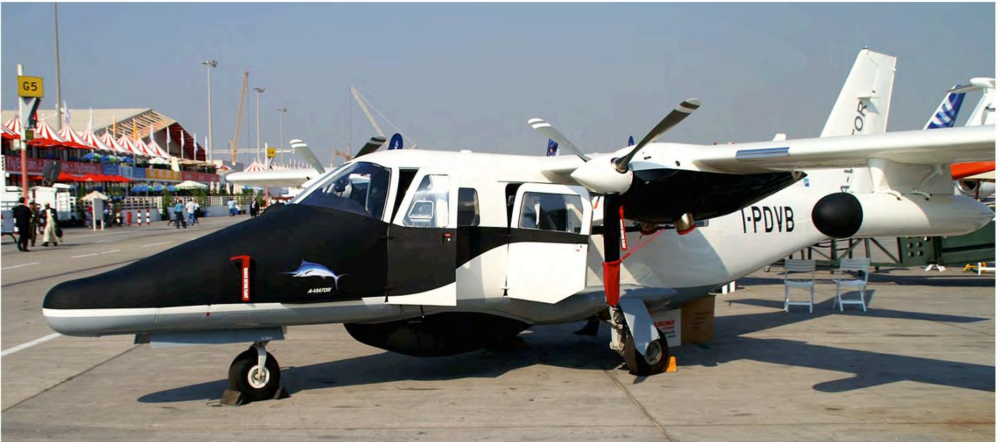
The aircraft shown here is a Vulcanair AP68TP-600, displayed at the Dubai Air Show in November 2009. While based on the Partenavia P68 Victor, it does not really look like it anymore. It is more similar to an Aero Commander or a Mitsubishi MU-2. Most apparent differences are the two engine exhausts at the bottom of the nacelles and the pointed nose. (Marco van Halum)
