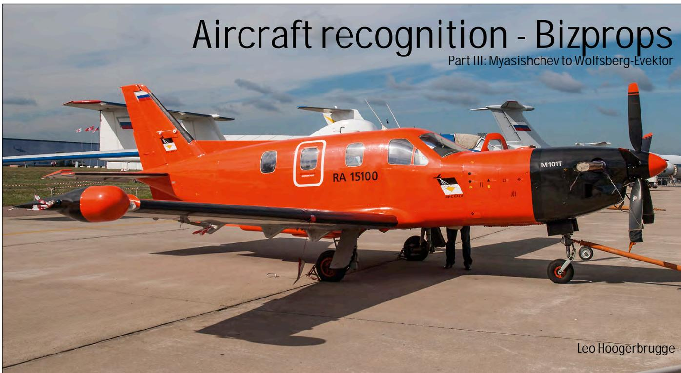
This is the Russian equivalent of the TBM series: the Myasishchev M-101T Gzhel. To keep them apart look at the nose gear and gear doors, and the engine cowling. (Zhukovsky, 19 August 2011)
