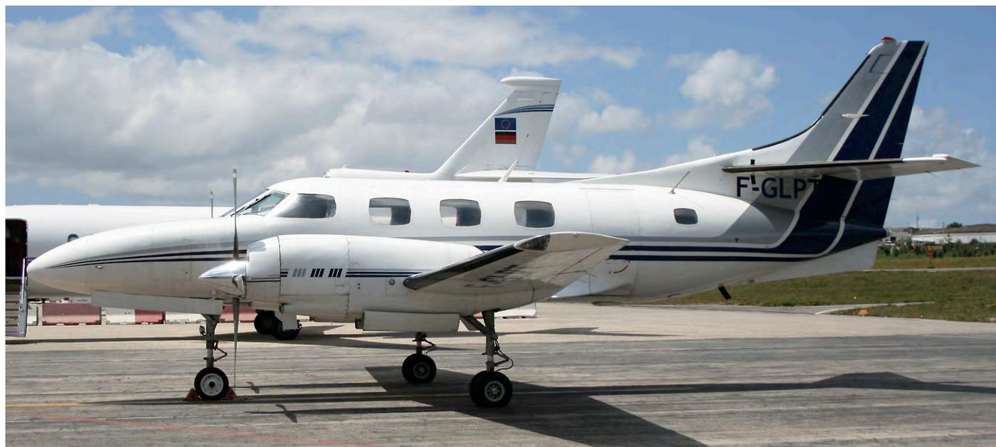
When you compare the Merlin IIA on the previous page to the Merlin III shown above, it seems like a completely different aircraft. In fact only the nose, gear, tail and engines nacelles are new. F-GIPT is an SA226T(B) Merlin IIIB, characterised by the small cabin window in the rear fuselage and the four-bladed props. (Lisbon, 12 May 2009, João Sa Pessoa)
