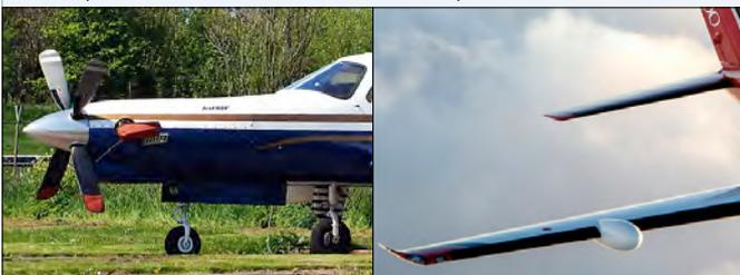
Piper developed a turboprop version of the Malibu, the PA-46-500TP Malibu Meridian. This spurred JetPROP to start converting existing Malibus, also with PT6A engines, resulting in the JetPROP DL and DLX. However, the engine cowling is different, with a single intake just aft of the prop. The improved M600 is recognised by the location of the weather radar. (Maastricht, 2 May 2010, John van Boven)
