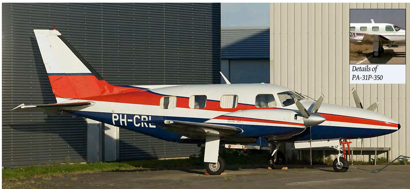
PH-CRL is a Pressurised Navajo, designated PA-31P. Compared to the original Navajo it has clearly smaller cockpit and cabin windows. Also the engine nacelles are shorter. The Piper PA-31P-350 Mojave (see inset) looks like the Pressurised Navajo, but has a larger cockpit side window and long nacelles.
