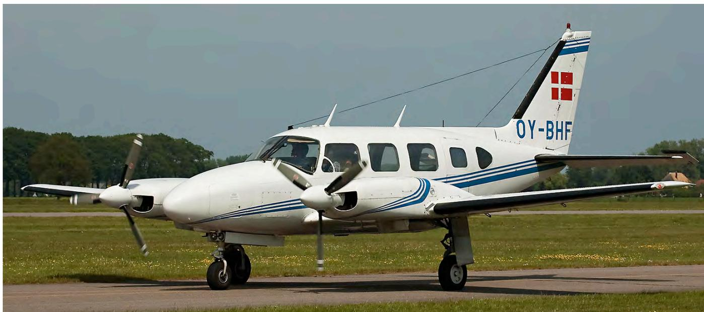
These two photos of PA-31 OY-BHF (Joost de Wit) and the Colemill Panther III conversion of PA-31-350 XA-UJM (Coert van Breda) show the main differences between the most-built PA-31s. Note the extra cabin window on the photo below, which is the main difference with the shorter PA-31 above. In addition note the four-bladed props and winglets which make XA-UJM a Colemill conversion.
