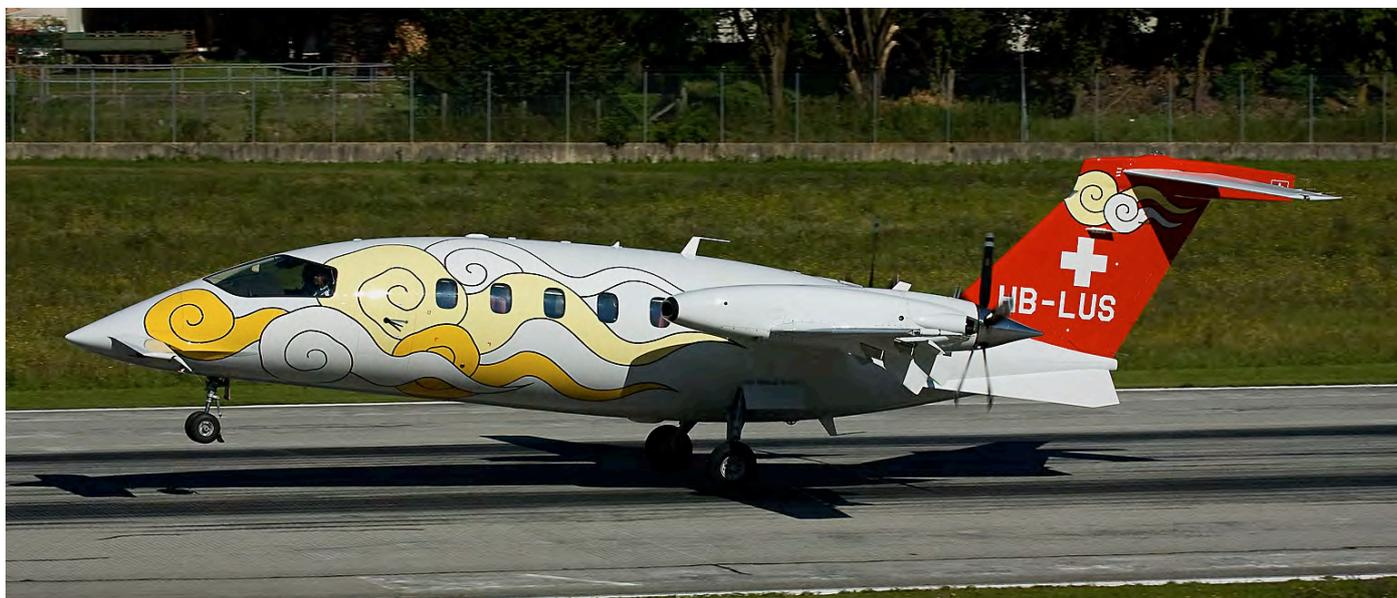
More than 200 Piaggio P180 Avantis have been built so far, so this canard bizprop is certainly more popular than the Beechcraft Starship. The Avanti has a so-called three surface configuration: a canard wing, main wing and a horizontal stabiliser (or actually a regular T-tail). The wing goes straight through the fuselage. (Lugano, 4 August 2010, Joost de Wit)
