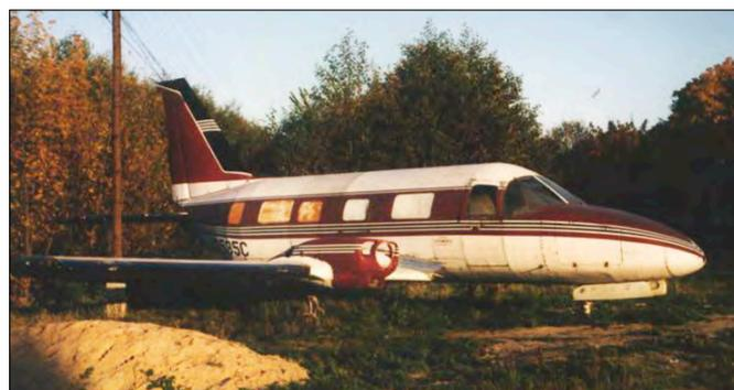
The Piper PA-35 looks like a “blown-up” Navajo, as it has a wider fuselage and a larger vertical tail. Just one such piston powered aircraft was built. (photo Hans Hoogers)
