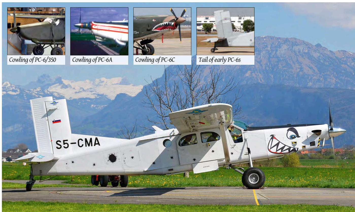
The Pilatus PC-6 (Turbo) Porter can best be recognised from other high wing tail wheel aircraft of similar size (like the DHC-2 Beaver) by its straight vertical tail and uniquely shaped cabin windows. The subtypes are essentially the same except for the engine and the dorsal fin. S5-CMA is a PC-6/B2-H4, characterised by its large dorsal fin and PT6A engine. The noses of other versions are shown on top. (Buochs, 9 April 2014, Stephan Widmer)
