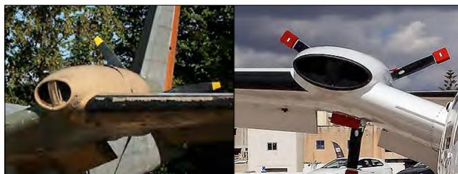
You can spot the difference between the P166AL1/ML1/S and P166BL2/CL2 by looking at the air intake: that of the first three is more rounded than that of the latter two.
