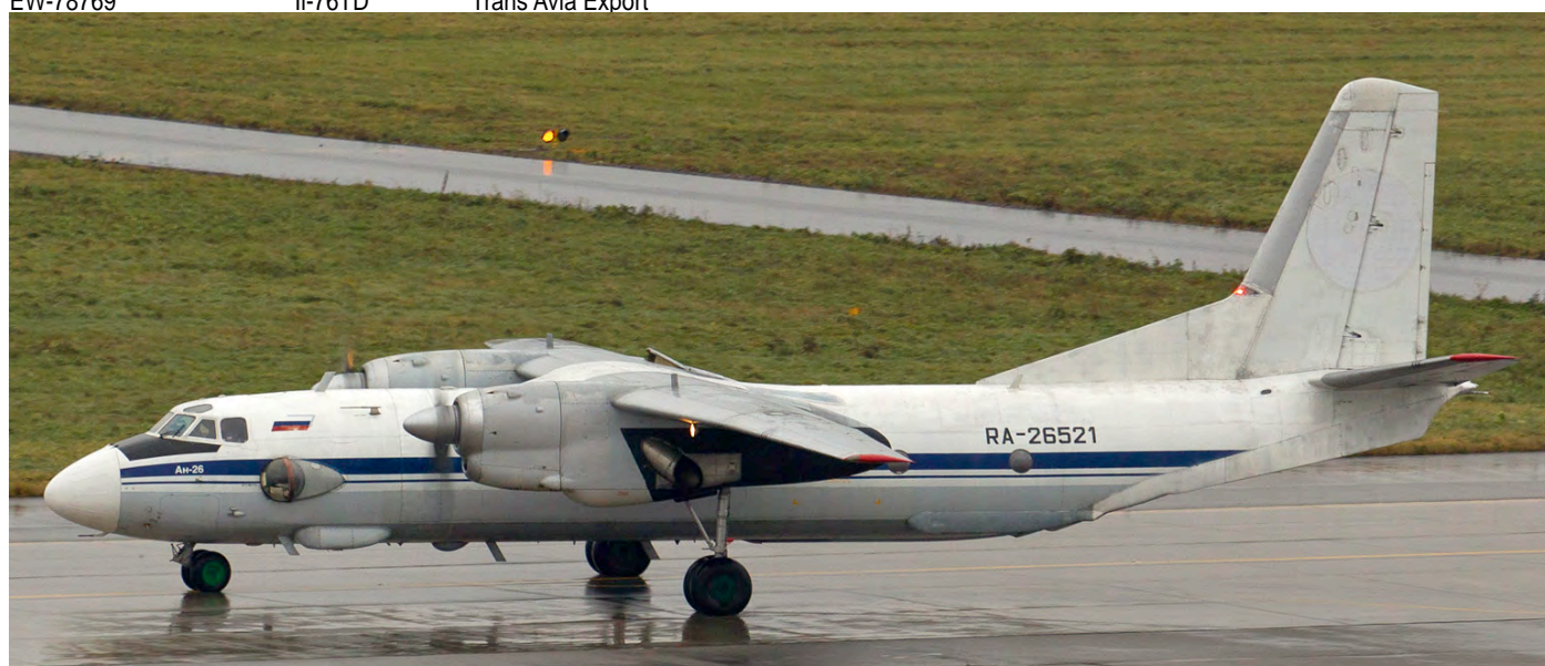
Antonov 26 RA-26521 is a version with an automatic calibration and navigation system, recognizable by the distinctive pod low on the forward fuselage side. The Antonov is listed in register with Lyotnyye Tehnologii as owner. (St. Petersburg-Pulkovo, 28 October 2016, André Alders)
