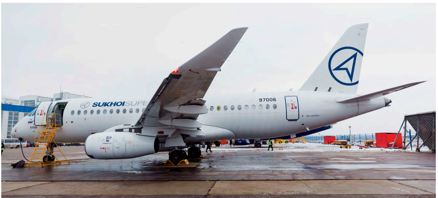
On the 21 December 2017, the Sukhoi Superjet 100 performed its first flight with the installed saberlets in Zhukovsky. This picture clearly shows the curves of the saberlets. (photo by Sukhoi Civil Air Company)
