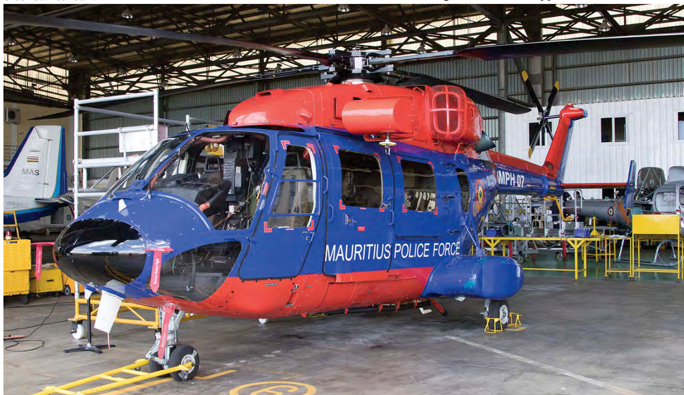
Most of us only know the Indian-made Dhruv helicopter fitted with skids. The Mauritius Police Force is one of the Dhruv CFW version fitted with wheels which looks rather different. (MPH-07, Mauritius-Seewoosagur Ramgoolam, 5 December 2017, Peter Heeneman)
