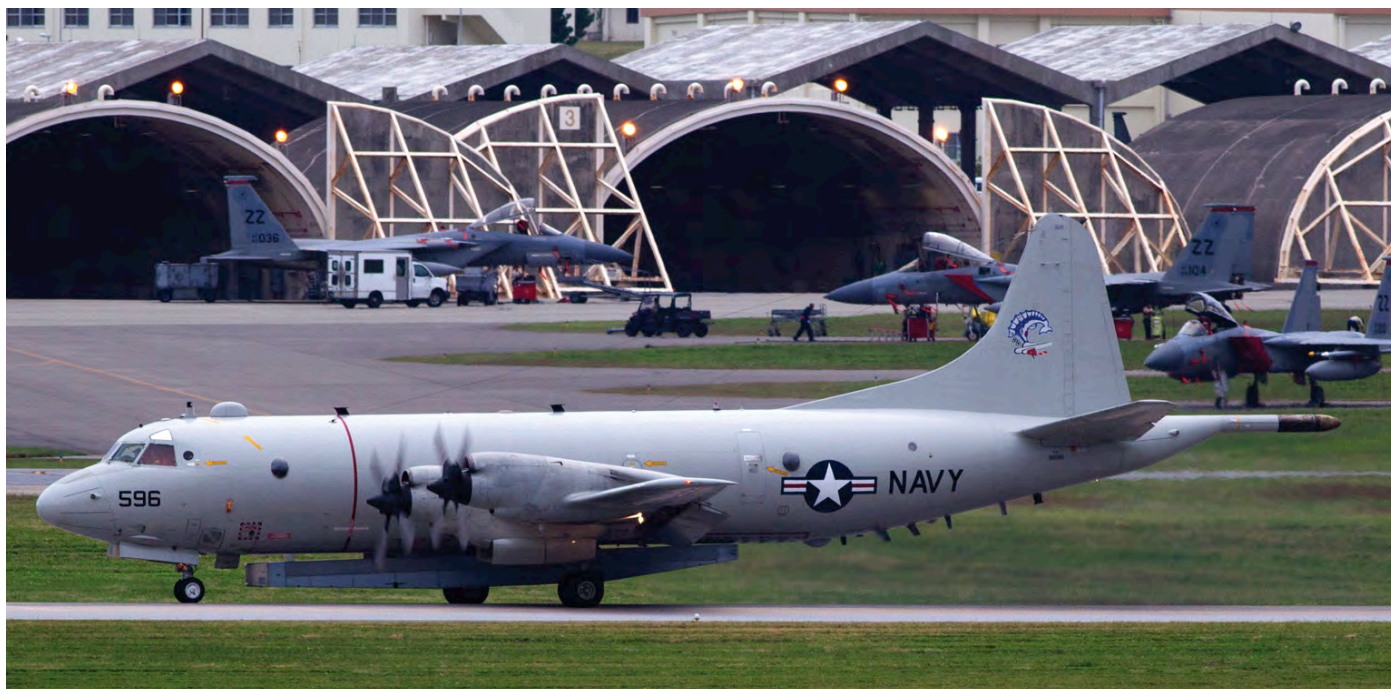
Seen at Kadena AB on 1 December 2017, is P-3C BMUP+ 161596 of VP-40 carrying a Raytheon AN/APS-149 Littoral Surveillance Radar System (LSRS). This unique radar system was designed to provide multi-function moving target detection and tracking and high resolution ground mapping at standoff ranges covering land, littoral, and water areas. With the introduction of the P-8, a new LSRS, called the Advanced Airborne Sensor (AAS) was developed for use on that specific airframe. Both the AAS and the AN/APS-149 adopt the active electronically scanned array (AESA) radar making it a unique system. (Kadena AB, 1 December 2017, Arnold ten Pas)
