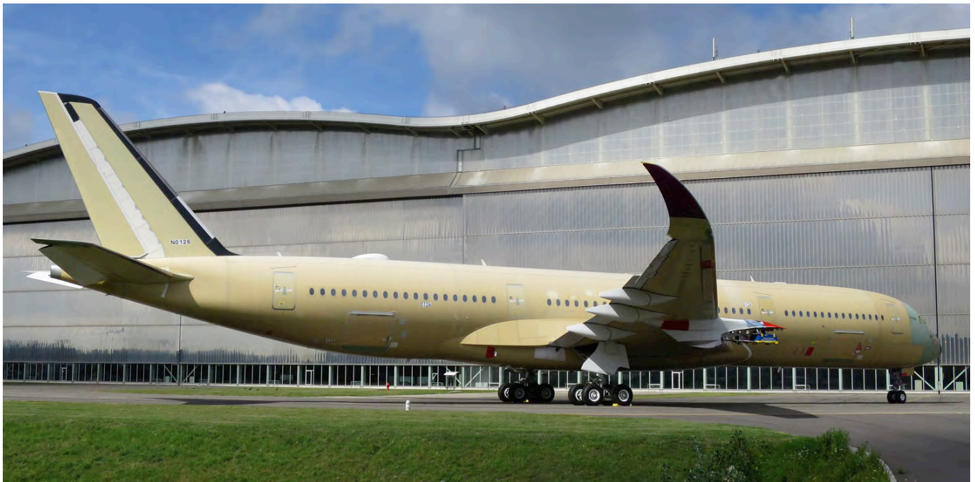
Newly built Airbus aircraft usually look like this A350-900, not in primer (which is usually greenish) but in this corrosive protective coating. Waiting outside a hangar at Airbus Toulouse for the mating of the engines, this A350 will be delivered as A7-ALX to Qatar Airways in the near future. (Gerben Hazebroek, 27 July 2017, Toulouse)
