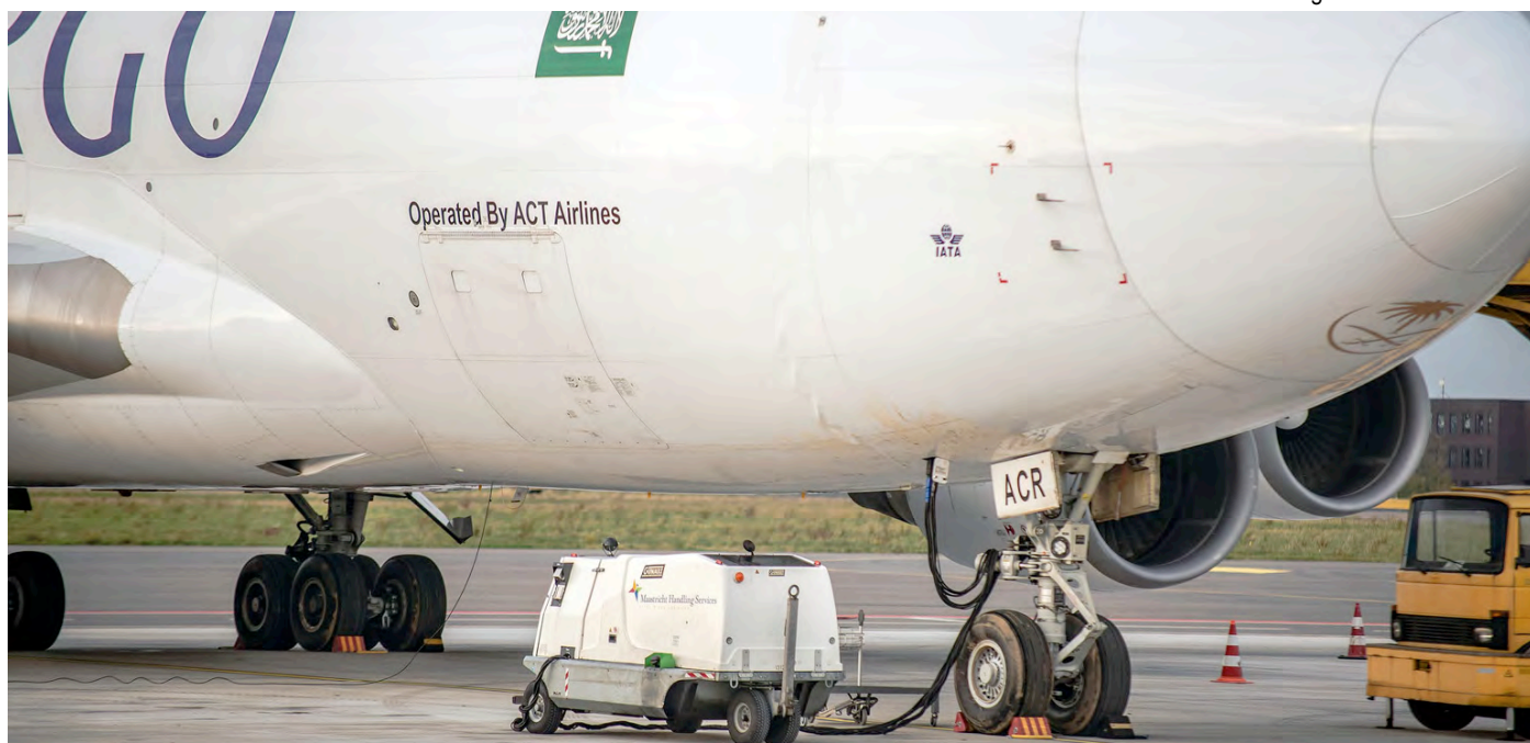
ACT Airlines Boeing 747 TC-ACR operated a cargo flight on behalf of Saudia Arabian Airlines when it suffered a runway excursion during take-off from runway 21. Initially there was no apparent damage (only muddy wheels and fuselage), but a wrinkle in the frame just aft of the nose wheel was later discovered. (Maastricht - Aachen, 14 November 2017, picmaickel.nl)
