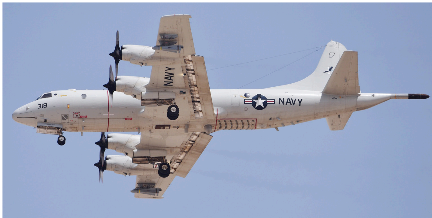
We do not regularly see Orions with underwing armament so this photograph of P-3C 162318 is worth publishing. The subhunter is seen here carrying AGM-65E Maverick missiles on its pylons. (Al Udeid, 21 March 2017, Taff Evans)
