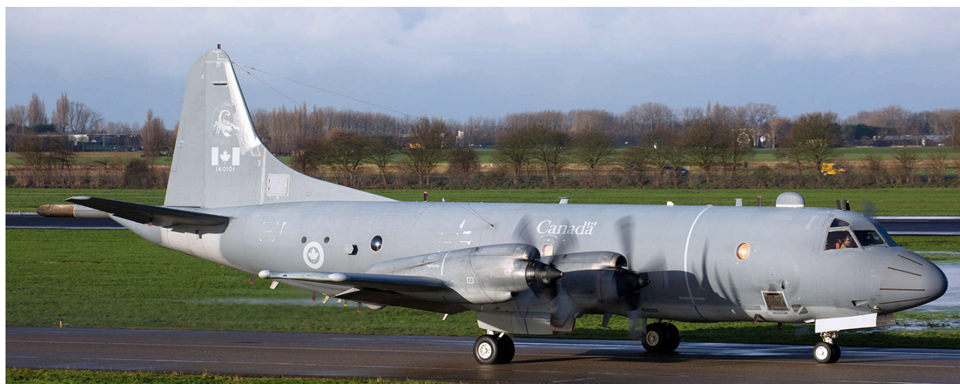
The CP-140 'Aurora' is a combination of the airframe of the P-3C Orion and the mission equipment suite of the S-3A Viking. The first flight of the Aurora was on 22 May 1979. 140101 is part of 14 Wing and based at Greenwood, Nova Scotia. It was caught on camera while on its way from Ali Al Salem Air Base, Kuwait back to Greenwood. (Rotterdam - The Hague, 16 December 2017, Peter Heeneman)
