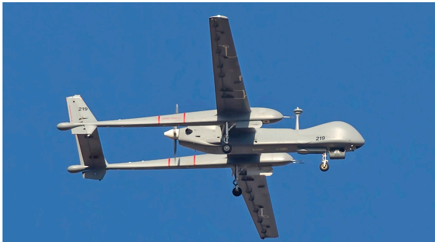
This will be most likely the future of military aircraft spotters, UAV's. The IAI Eitan "Steadfast", also known as Heron TP, is an unmanned reconnaissance aircraft developed in Israel by the Malat division of Israel Aerospace Industries. The aircraft is a newer version of the IAI Heron. (Tel-Nof/Ekron AB, 6 November 2017, Dino van Doorn)
