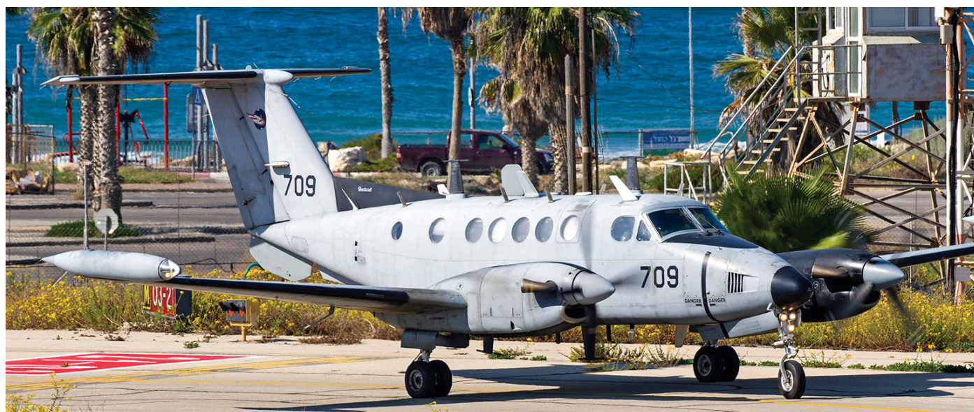
Many variants of the Beech 200 light transporter are in use with the Israel Air and Space Force and they all are based at Sve Dov. The five Beech B200CT Zufit-3's, like this 709 of 135 squadron, are used for IMINT duties. (Tel-Aviv/Sde Dov, 6 November 2017, Dino van Doorn)
