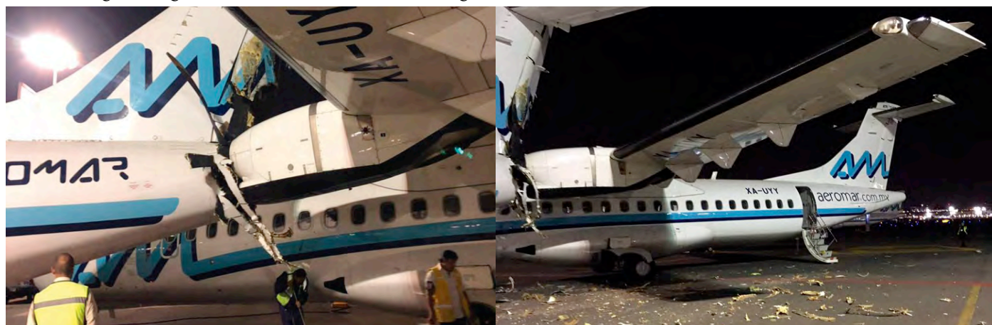
Aeromar Airlines can submit a big claim with its insurance company, after two of their ATRs collided with each other. ATR72 XA-UYU was engaged in an engine test run when the aircraft jumped the chocks and hit parked ATR42 XA-UAV. The carnage it created is seen on these two pictures, taken shortly after the incident on 29 March 2018. (AviationPhoto Mexico)
