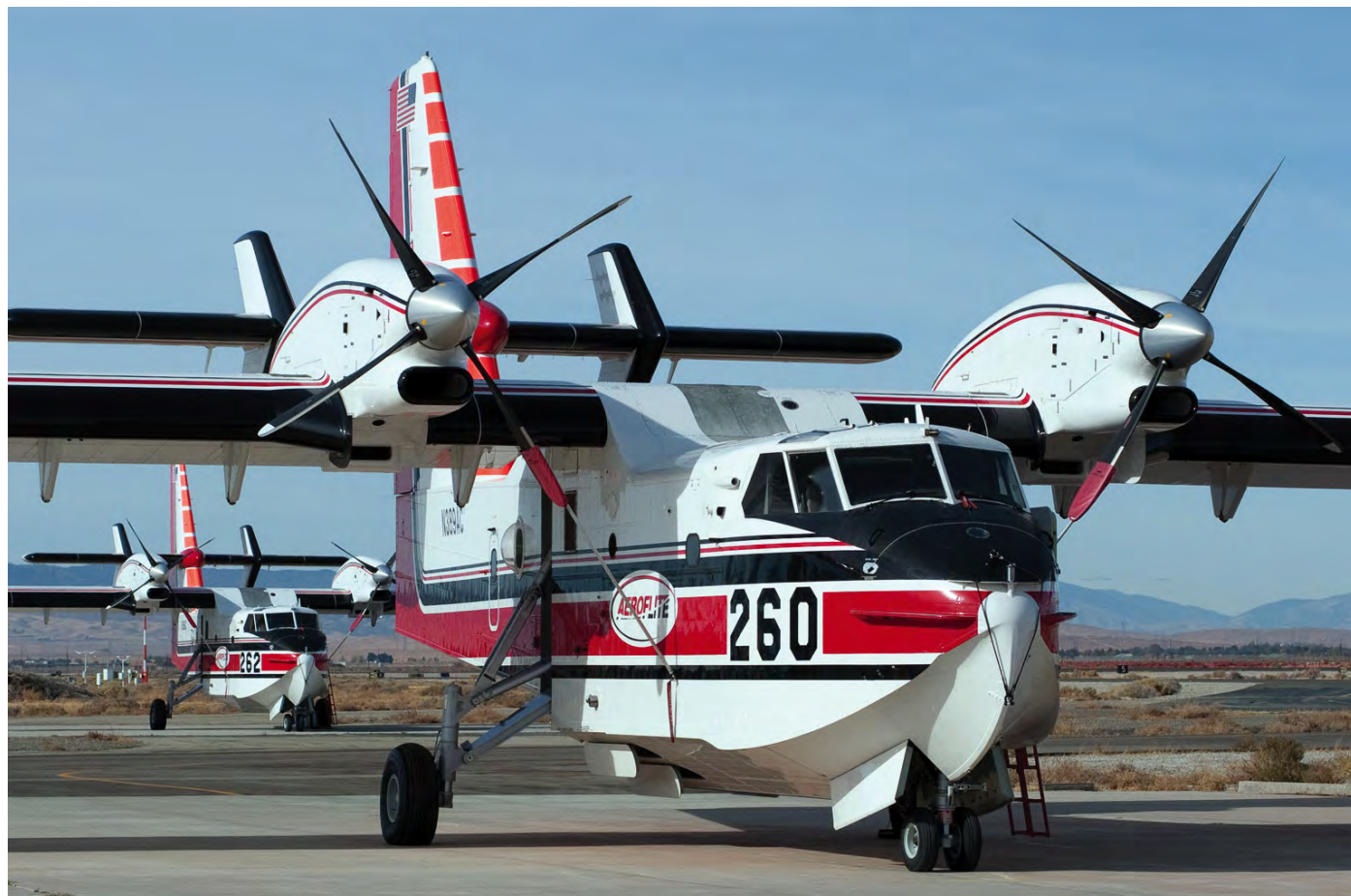
N389AC is one of four Viking CL-415 water scooping aircraft operated by Aero-Flite. The amphibious aircraft was added to the fleet in 2013. (General William J. Fox (CA), 20 November 2017, Joost de Wit)
