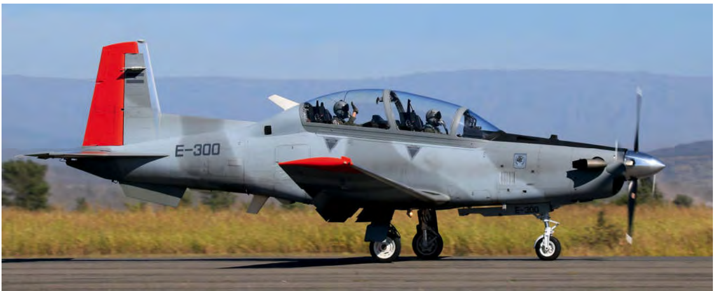
The successor of the Tucano is the Beechcraft T-6C+ Texan II. It differs from the standard T-6B in having wings that are plumbed for the carriage of auxiliary fuel tanks. The enhanced T-6C+ variant procured for Argentina (and previously Mexico) is also capable of carrying up to a payload of 1,415 kg of external stores. The FAA requested 24 aircraft but this was brought down to only twelve of which until now only four aircraft are delivered. The last one should be delivered in 2022. (Córdoba, 26 March 2018, Leonard van Teeffelen)
