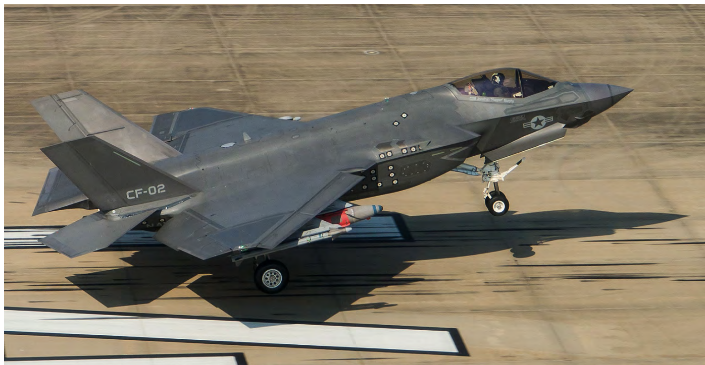
CF-2 completed the final SDD flight at Naval Air Station Patuxent River (MD), on 11 April 2018. The F-35C from the F-35 Pax River Integrated Test Force completed a mission to collect loads data while carrying external 2,000-pound GBU-31 Joint Direct Attack Munitions (JDAM) and AIM-9X Sidewinder heat-seeking missiles.
