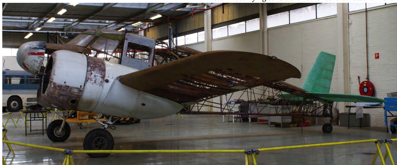
As can be seen, the Cessna Bobcat in the museum has seen some progress in its restoration, as the stationary vertical and horizontal parts of the tail have been covered with fabric. Once restored, the type will be a rare exhibit in Europe.
