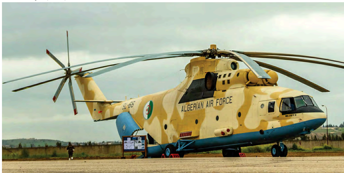
The big star, literally, of this year Portes Ouverte at Chlef Air Base, was the recently delivered Mi-26T-2. Algeria ordered six of these giants in February 2014 and eight more in June 2015. The SL-66 on the photo is equipped with the President-S protection system. The total system includes a laser illumination detector, ultraviolet missile approach warning system, an electro-optical electronic warfare system, a command and control system and decoy flares. (Chlef, 29 March 2018, Kingvarg)
