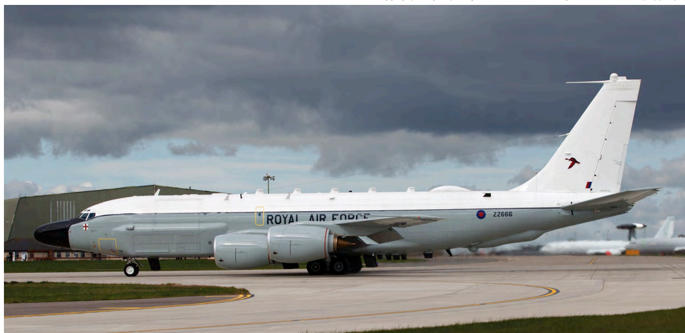
The United Kingdom bought three former USAF KC-135R aircraft for conversion to RC-135W Rivet Joint standard under the Airseeker project. The ZZ666 was the final aircraft which was delivered in June 2017 to 51sq (Waddington, 25 April 2018, Marcel J. van Bielder)
