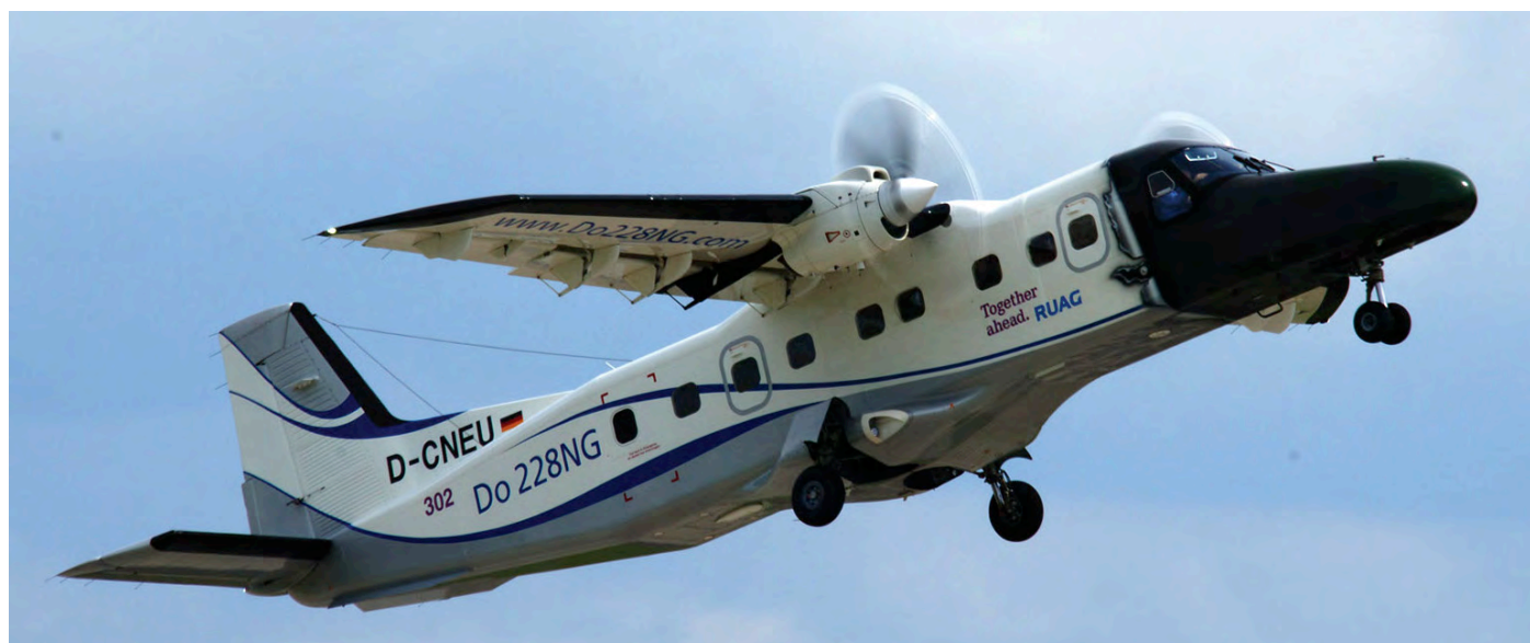
Dornier Do228-212NG D-CNEU is a prototype, developed by RUAG Aerospace, of the unpressurized STOL transport Do228-200, with glass cockpit and new 5-blade propellers. (Berlin-Schönefeld, 27 April 2018, Rob Vogelaar)
