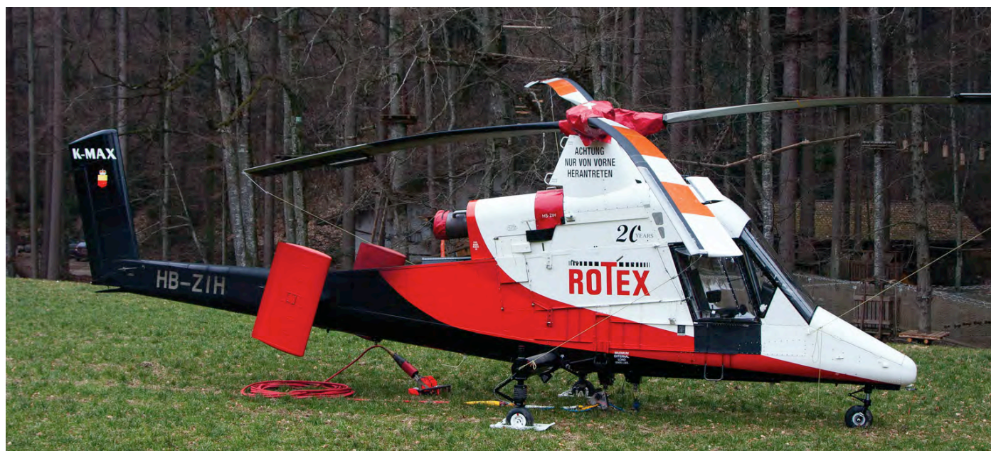
While a bit of an ungainly sight, the Kaman K-1200 K-MAX is quite a unique helicopter with its intermeshing rotors. HB-ZIH is one of three operated by Rotex and was built in 1997 during its original production run. The production line was revived in 2017. (Wilderwill, 7 February 2018, Michiel van Herten)
