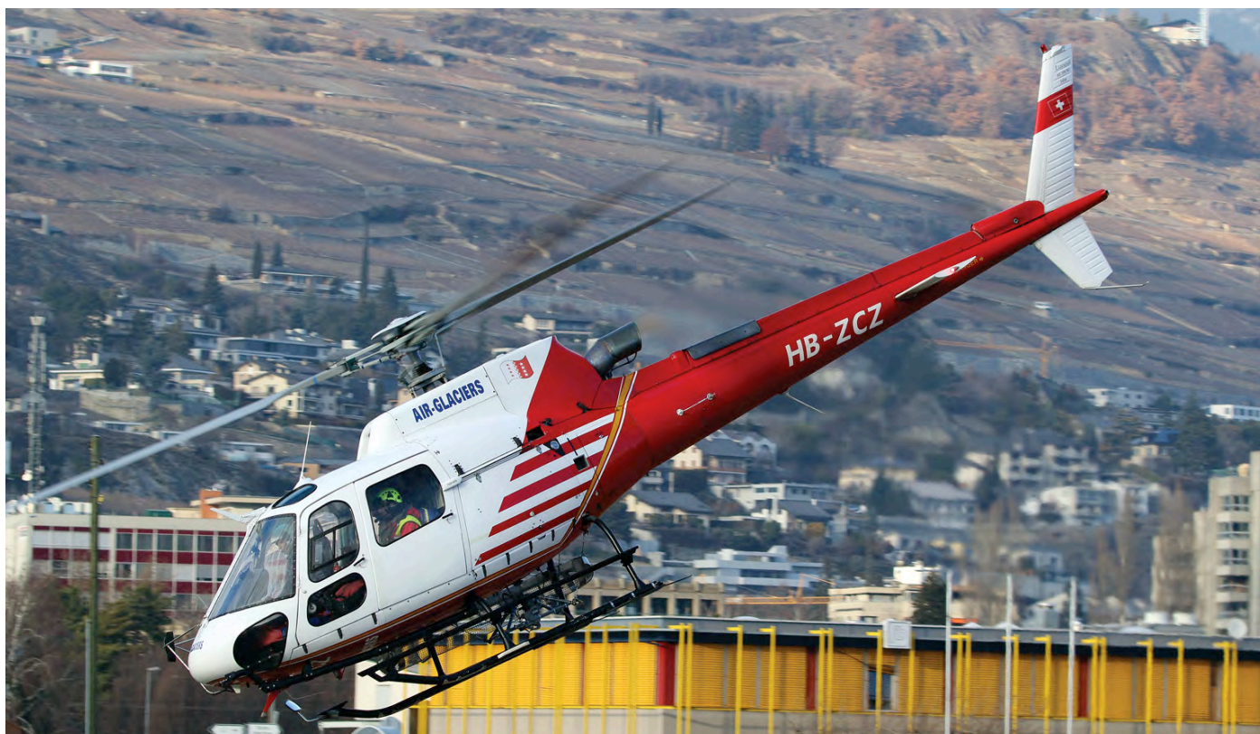
Air Glaciers the second Swiss helicopter operator after Heliswiss and was founded in 1965. The company is based in Sion and operates around fifteen helicopters, a few King Airs and a PC-6. HB-ZCZ is one of a few AS350s operated by Air Glaciers (Sion, 8 February 2018, Michiel van Herten)
