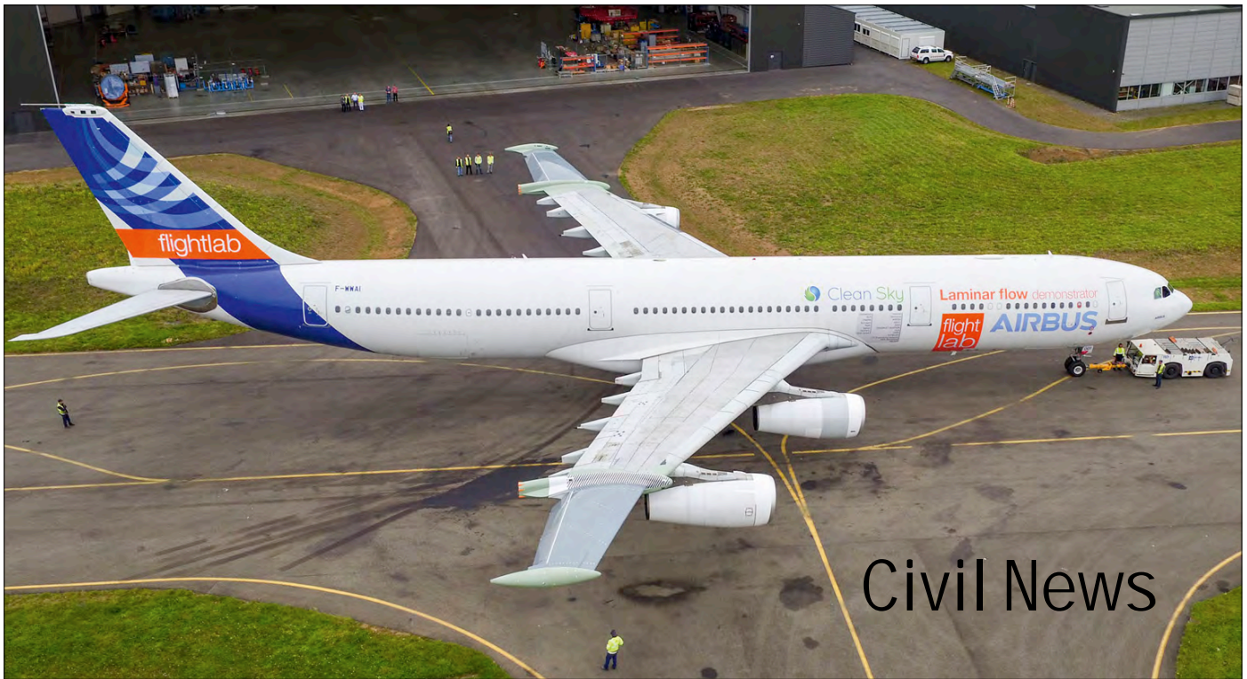
On 26 September, the Airbus A340 laminar-flow “BLADE” test demonstrator aircraft made its first flight with the new wingtips. The Airbus test bed F-WWAI is the first A340 ever built (MSN 1) and has never been delivered to a commercial operator. (@Airbus, D-Vicart, September 2017)
