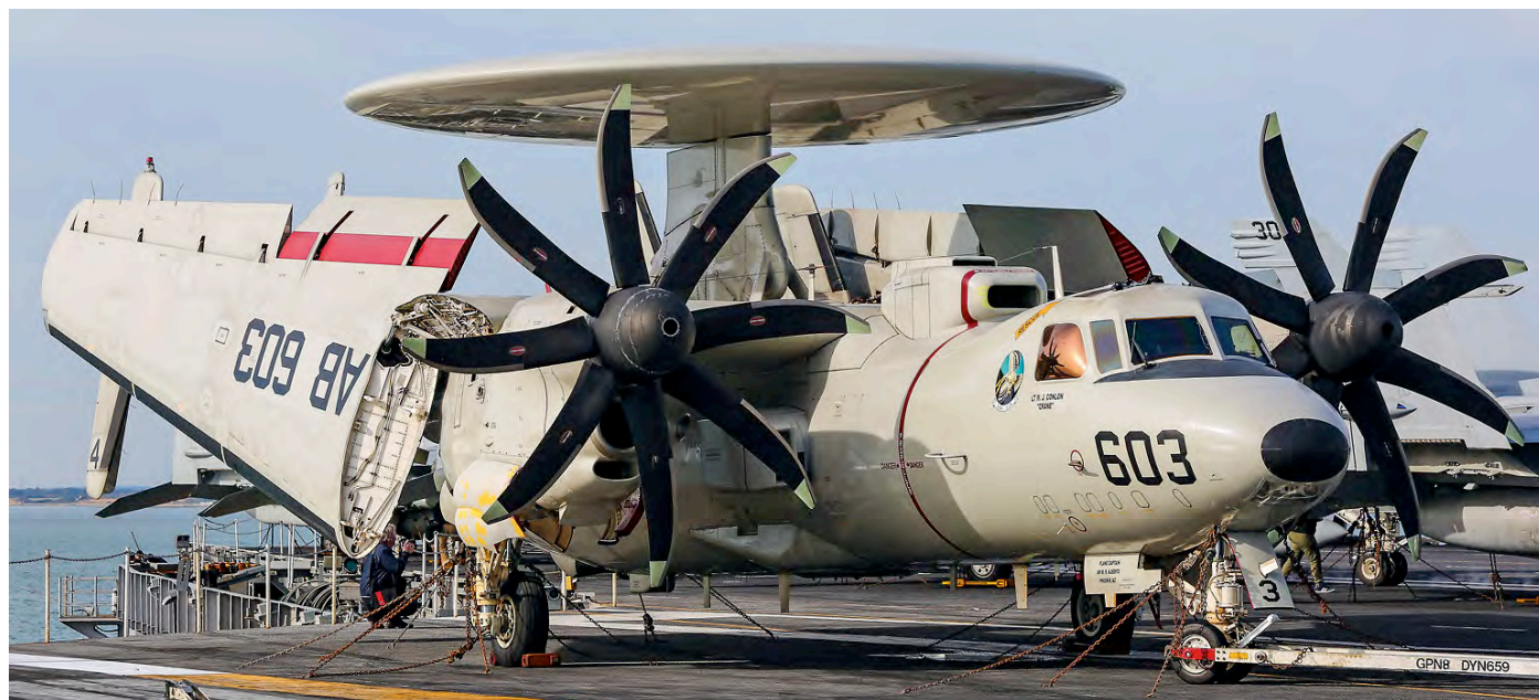
With its eight-bladed propellers in evidence, E-2D 168594/AB-603 from VAW-126 'Seahawks' enjoys the bleak sun. (onboard CVN-75, 7 October 2018, Mark Rourke)
