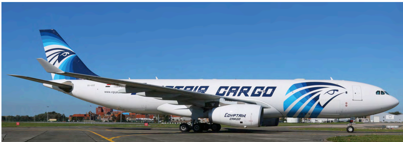
Airbus SU-GCE was delivered to EgyptAir as a passenger aircraft in 2004. Previously using the Airbus A300-600F for cargo flights the airline signed an agreement in December 2014 for the conversion of two A330-200s plus two options. SU-GCE was re-delivered to EgyptAir as A330-200(F) on 4 August 2018. Nik Deblauwe photographed the aircraft on its first visit to Ostend on 27 September 2018.
