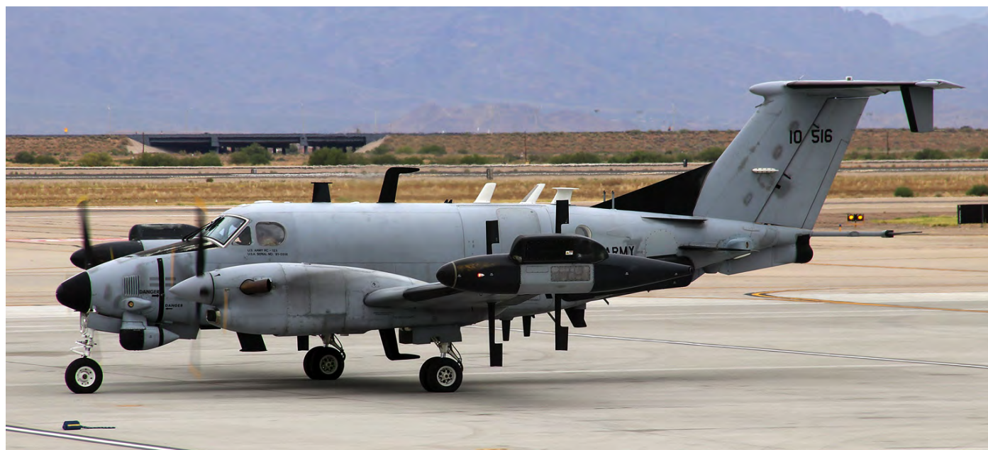
The Beechcraft RC-12 Guardrail is an airborne signals intelligence collection platform and used by the US Army. This RC-12X with serial 91-00516 belongs to the 204th MI Bn and is based at El Paso/Biggs Army Airfield (Fort Bliss) Texas. (Phoenix-Mesa Gateway (AZ), 19 May 2019, Ramon Berk)
