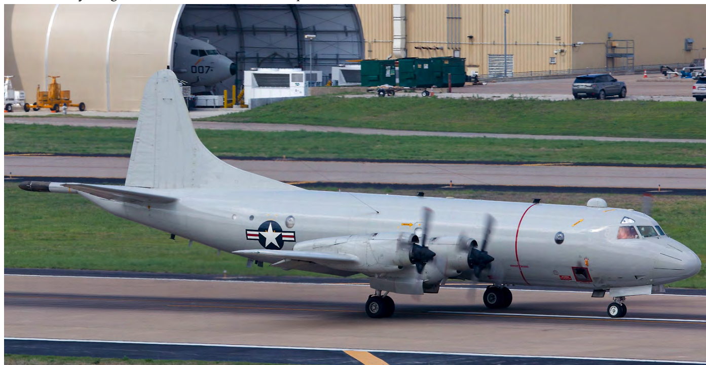
Without its external surveillance radar, only its anonymity and the small roof antennae and radar bulge give this P-3 Orion away as a special missions aircraft. We refer to the item on BUPERS for more information. (Dallas-Love Field, June 2019, Garrett Heller)
