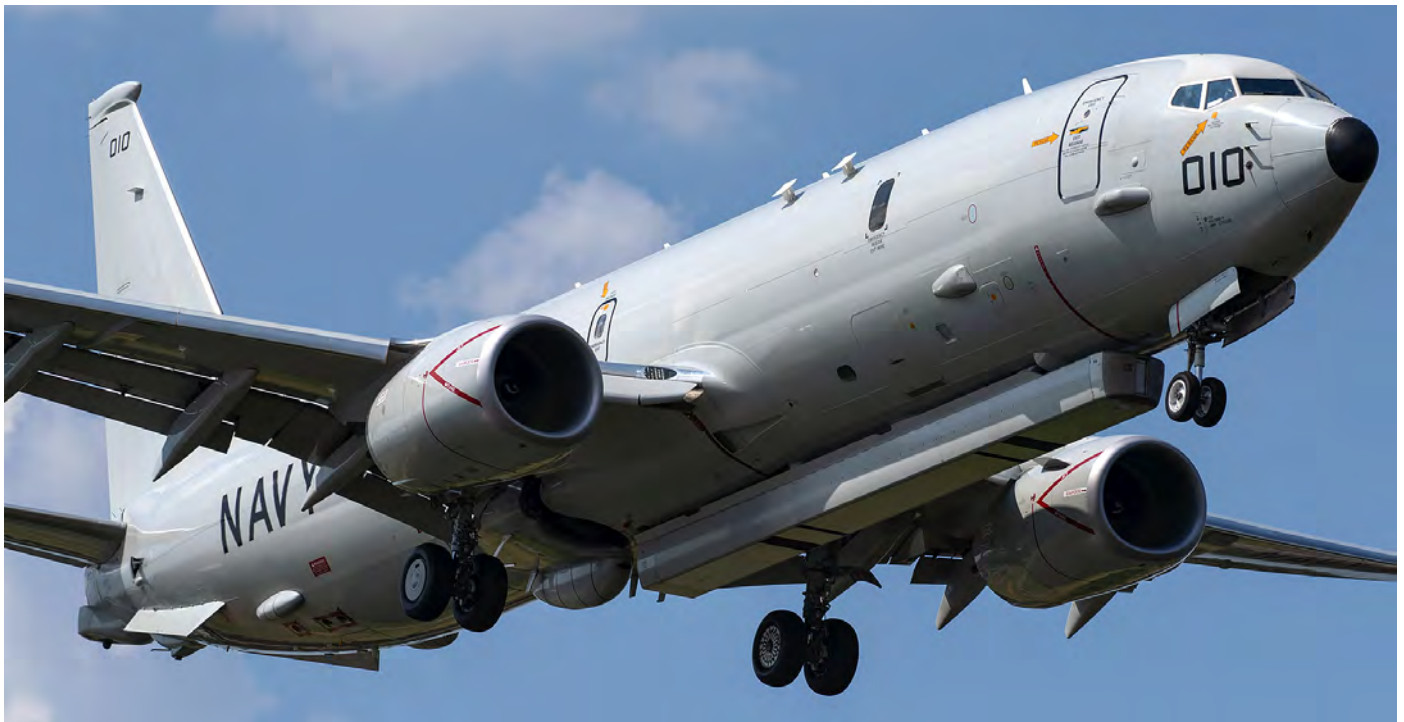
US Navy P-8A Poseidon BuNo 169010 of the Naval Air Systems Command-Flight Support Detachment is seen approaching runway 13R at Dallas-Love Field after a sortie over the Gulf of Mexico. Attached underneath the fuselage is a Raytheon Advanced Airborne Sensor (AAS). The unit's mission is shrouded in secrecy, but it has been rumoured as a (mainly) drug interdiction unit. (7 August 2019, Dylan Phelps)
