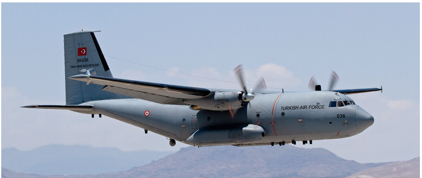
C-160D Transall 69-036 has been modified with the Gören-1 upgrade, explaining the huge number of extra antennas and other equipment. It could be seen during Anatolian Eagle 2019 at Konya. (26 June 2019, Dino van Doorn)
