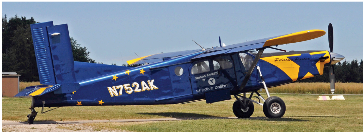
N752AK is operated by Skyservice Altmühlthal for Skydive Colibri, based at Thalmässing airfield in southern Germany. It is a PC-6/B2-H4, c/n 752, the former Austrian Air Force PC-6/B2-H2 3G-EA. Note that the subtype has changed from when it was 3G-EA, as can be identified by the upturned wingtips. (Thalmässing, 6 July 2019, Martin Bach)
