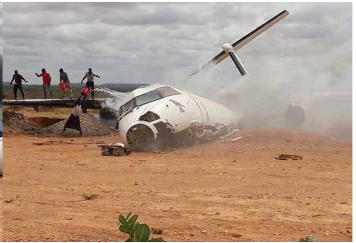
A donkey was to blame for the loss of this Bluebird Aviation Dash 8-400 5Y-VVU, after the crew had to deviate for the poor animal and subsequently the DHC-8's landing gear collapsed. Poor (as in non existent) fire service at the airport of Beledweyne meant the Dash was a write off, having been destroyed by fire. (Beledweyne Haji-Sheikh Mahmud Hasan, 14 July 2020, JACDEC)
