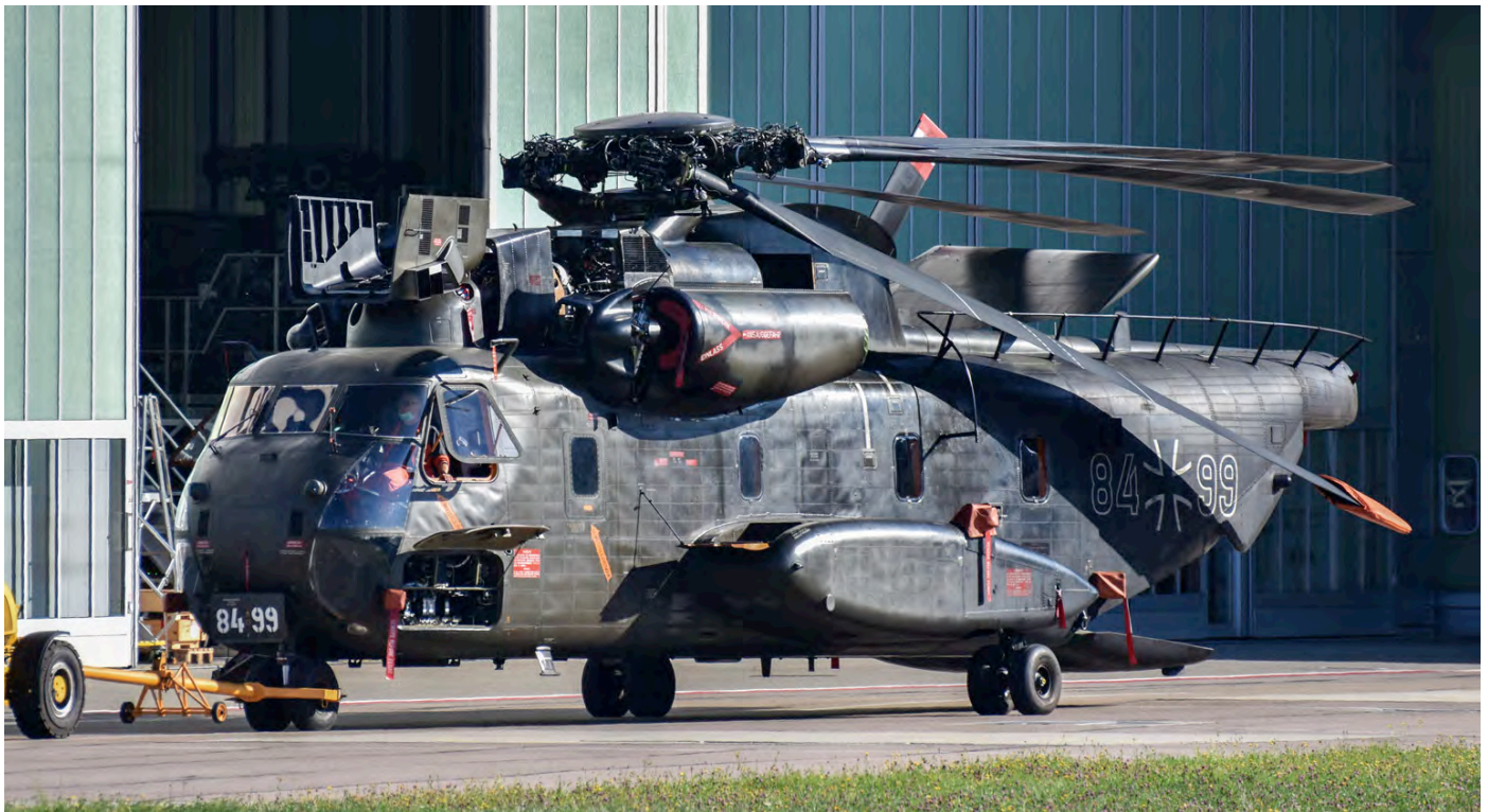
The CH-53s are being upgraded at Airbus Helicopters, Donauwörth and receive new avionics. CH-53GA 84+99 is seen here being towed from one hangar to another in folded status. (Donauwörth, 26 June 2020, Wim Sonneveld)
