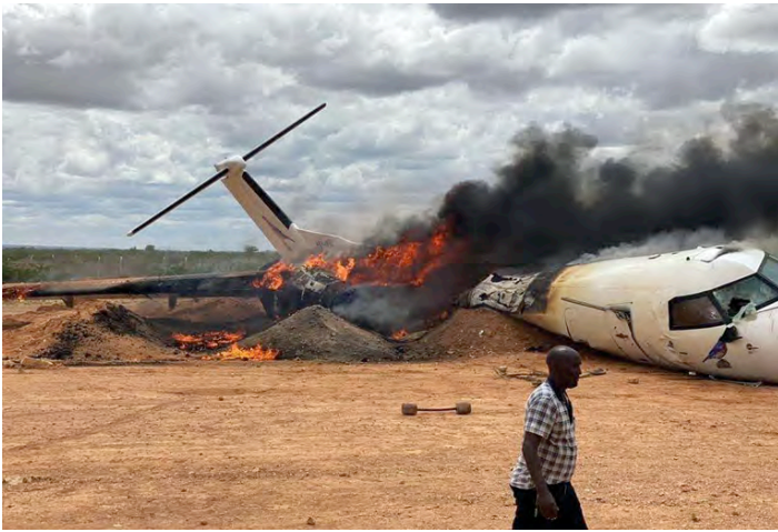
A donkey was to blame for the loss of this Bluebird Aviation Dash 8-400 5Y-VVU, after the crew had to deviate for the poor animal and subsequently the DHC-8's landing gear collapsed. Poor (as in non existent) fire service at the airport of Beledweyne meant the Dash was a write off, having been destroyed by fire. (Beledweyne Haji-Sheikh Mahmud Hasan, 14 July 2020, JACDEC)
