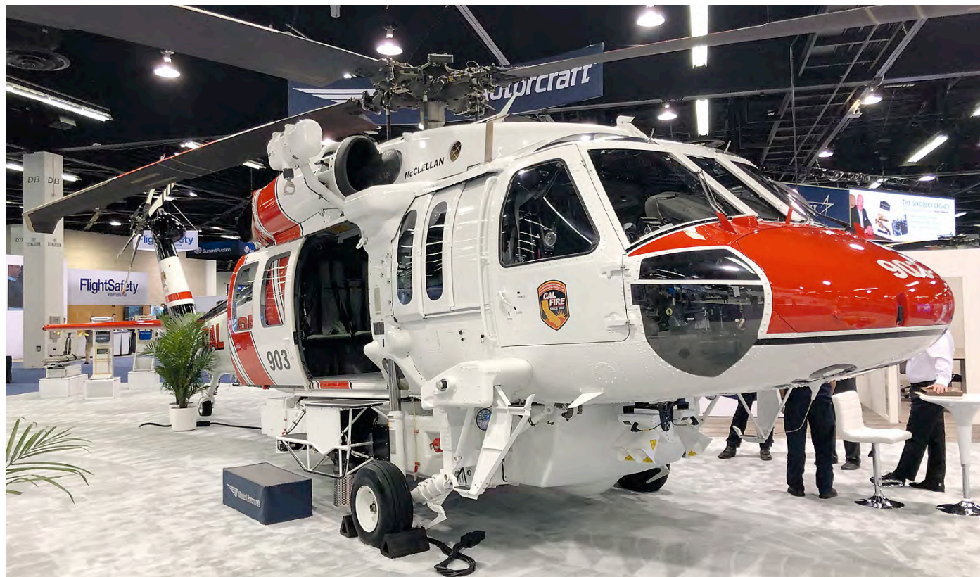
Compared to the well-known US Army Blackhawk, the new Fire Hawk has a heavily modified exterior. The reconfiguration into an aerial firefighting platform has necessitated an extended landing gear way to the 1,000 gallon firefighting tank and the retractable snorkel system. Photo of N483DF (Tanker #903) was made by Lukas Hollnsteiner at Anaheim (CA) on 28 January 2020.
