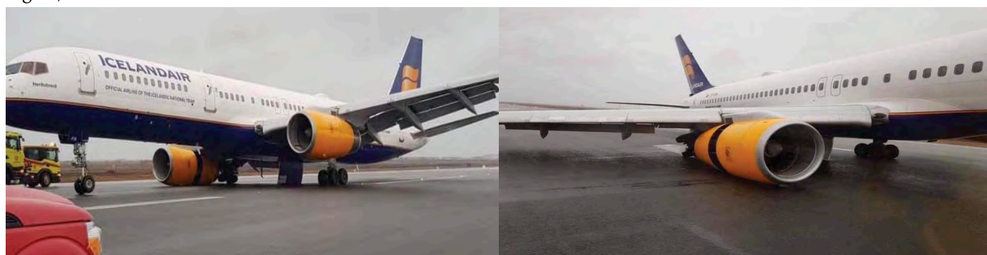
Icelandair Boeing 757 TF-FIA, operating flight FI529 from Berlin-Tegel, suffered a right main gear collapse during landing at Keflavik. The accident happened on 7 February 2020 and is most probably caused by very strong cross winds.
