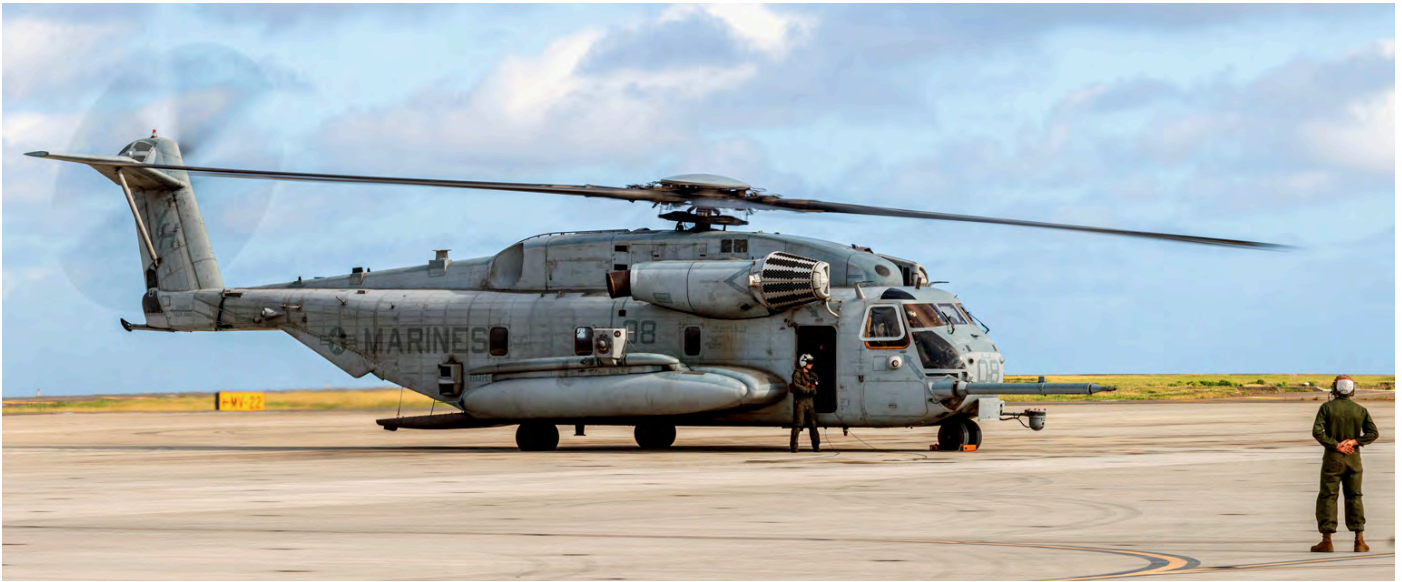
Crew members attending CH-53E 162005/YH-08 with its seven blade, 24m (79ft) diameter rotor, driven by three engines.
