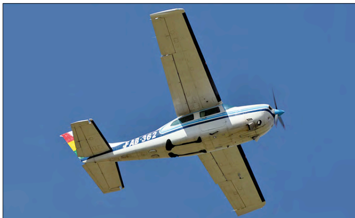
The Cessna Centurion is a popular aircraft for skydiving, retractable gear, no wing struts. GAC34's FAB-362, was impounded as PT-WEL. (Santa Cruz-El Trompillo, 12 October 2013, Wim Sonneveld)
