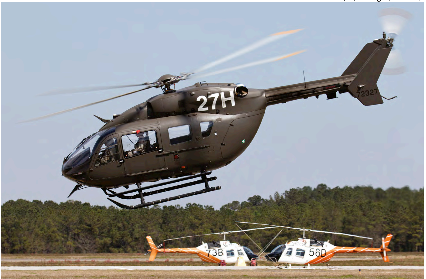
The United States Army decided to replace the OH-58A/C Kiowa and TH-67A Creek helicopters in use as training helicopters at the Fort Rucker, Alabama, complex by the UH-72A Lakota. Some minor modifications were made to the helicopters for this new role, but from the outside they look the same as a regular 'slick' UH-72A (albeit minus the external hoist on the right-hand side). The biggest give away is the large white buzz number applied to the fuselage of all helicopters in use for training purposes at Fort Rucker. (14-72327, Fort Rucker, Alabama, 16 March 2017, Tony Osborne)
