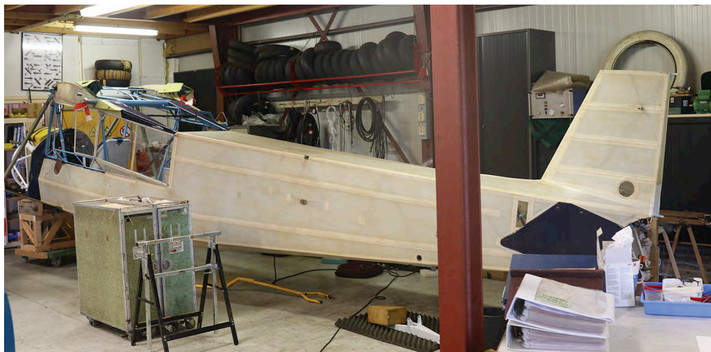
This MS505, N156EB/752, is under restoration at the Stichting Vroege Vogels hangar at Lelystad. It was built as MS500 for the French Air Force and after it became F-BAYE it was converted to MS502 and later to MS505. (19 September 2020, Otger van der Kooij)
