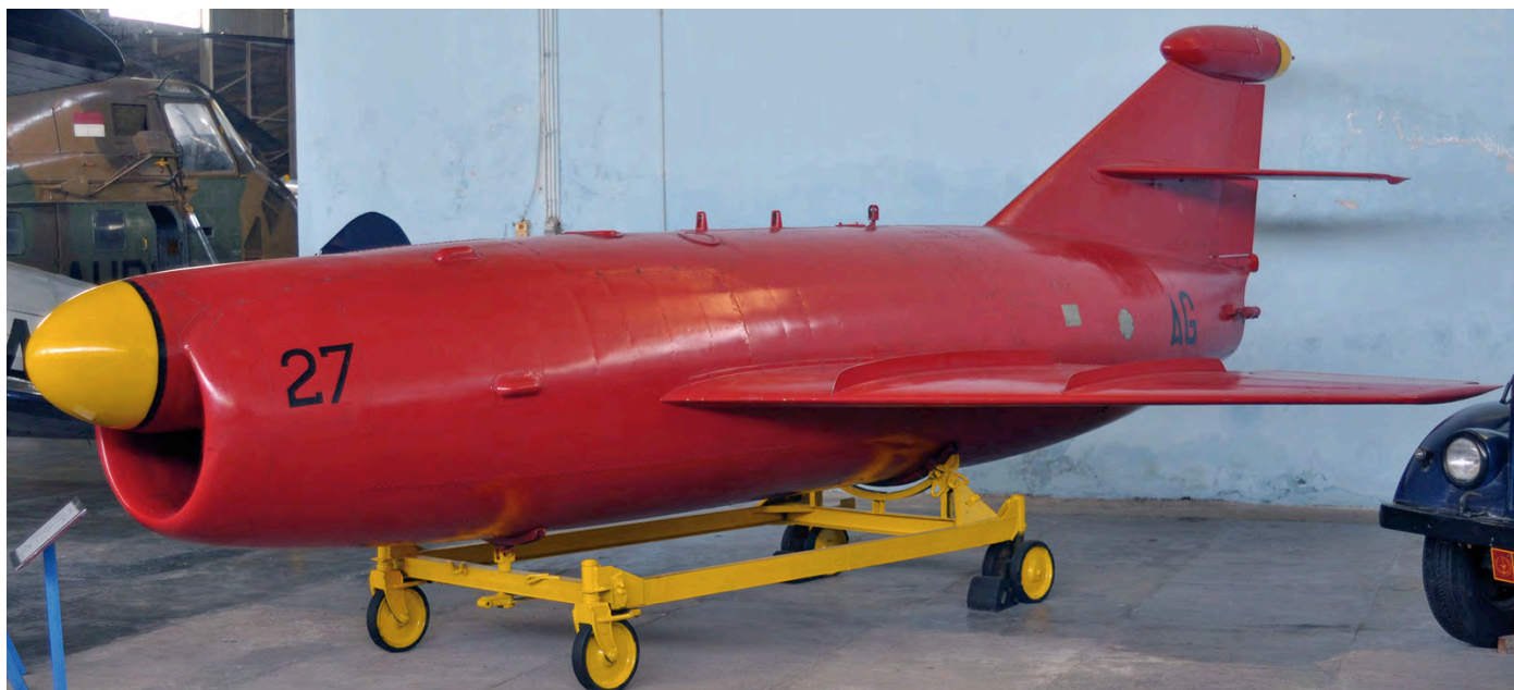
The business end of the Tu-16KS: The Raduga KS-1 Komet (NATO reporting name: AS-1 Kennel) air-launched short range air-to-surface missile. They were never used in anger by AURI. (Yogyakarta, 21 August 2009, Marco Pennings)
