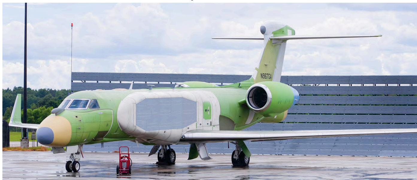
Heavily modified Gulfstream G550 N967GA (c/n 5567) was photographed at its place of birth Savannah-Hilton Head International (GA). It already rolled off the production line in late 2017 and has since been modified to a Conformal Airborne Early Warning (CAEW) aircraft. (26 August 2021, Dohwan Kim)
